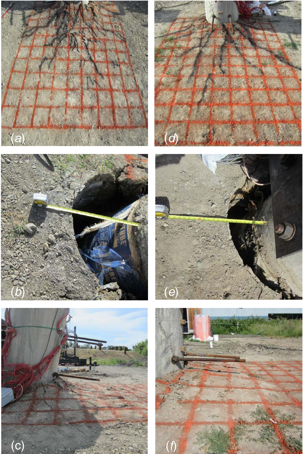
Figure 7.1: Photos at the end of the loading tests showing: (a) crack patterns, (b) gap behind the shaft, and (c) side view of the shaft for MIR with applied displacement of 523 mm (20.6 in), and (d) crack patterns, (e) gap behind the shaft, and (f) side view of the shaft for HSIR with applied displacement of 305 mm (12.0 in).
