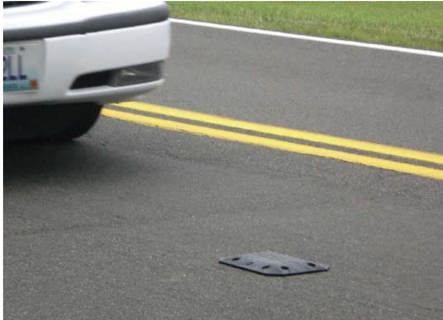
Figure 3.2: Placement of Portable Traffic Analyzer by Nails (Vaisala 2012)
