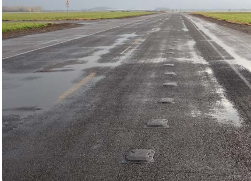
Figure 4.1: Sensor Layout on First Day of Sensor Testing
