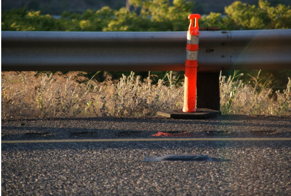
Figure 3.3: Placement of Portable Traffic Analyzer using Adhesive Tape
