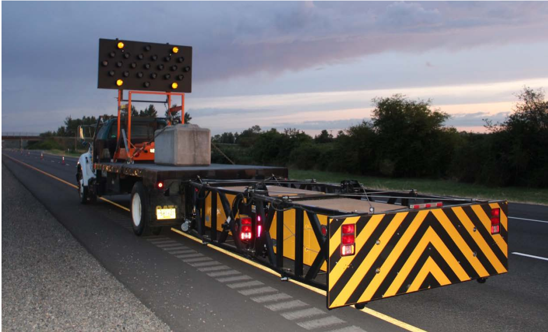
Figure 2.8: Truck Mounted Attenuator and Sequential Arrow Board
