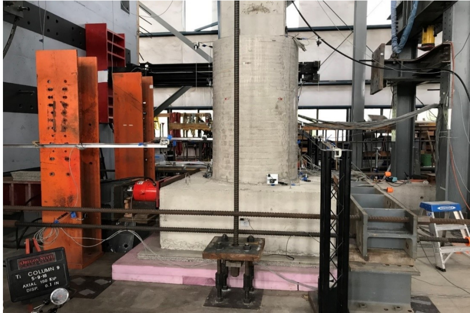
Figure 3.72: Photograph of setup details for spread footing
