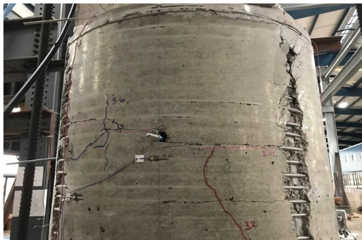
Figure 4.10: Specimen R-S-R-LTi-135: Reduced visual distress near the TiAB hooks (South face) at the end of testing
