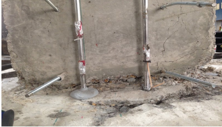
Figure 4.31: Specimen RS-T-R-LTi-90: Concrete cone pulled at top of the footing (shell removed after testing)
