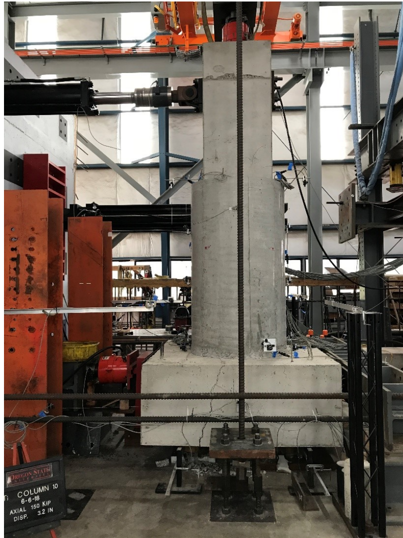
Figure 4.23: Specimen R-S-R-LTi-90-Pile: Column at the end of testing (at approx. 4% total drift level), limited cracking in column, large cracks in footing
