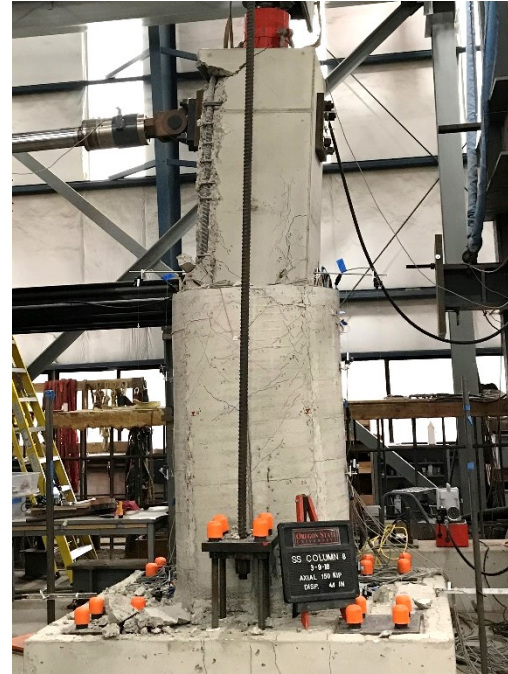
Figure 4.17: Specimen R-S-R-LSS-90: Critical observations at 4.4 in (approx. 4.4%) drift level: a) Spalling of cover concrete on South side above the retrofit shell, b) Column cranking about the top of the retrofit shell
