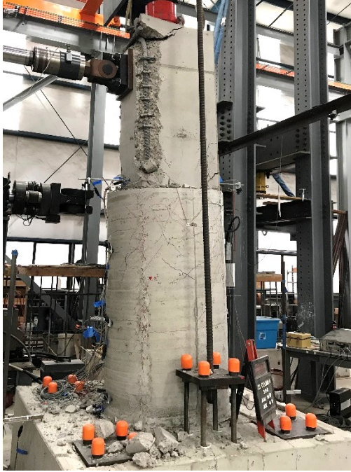
Figure 4.17: Specimen R-S-R-LSS-90: Critical observations at 4.4 in (approx. 4.4%) drift level: a) Spalling of cover concrete on South side above the retrofit shell, b) Column cranking about the top of the retrofit shell
