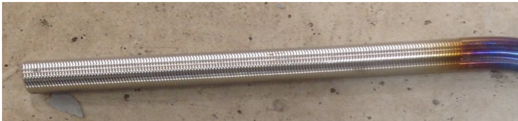
Figure 3.35: Surface deformations on extension of 90° hook on TiAB ligaments
