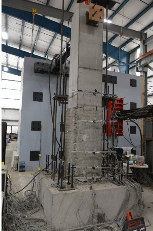
Figure 4.28: Condition of specimen R-T-R-LTi-90: corner spalling of concrete shell and cracking at TiAB ligament hook locations at end of test (maximum 8.2% drift)
