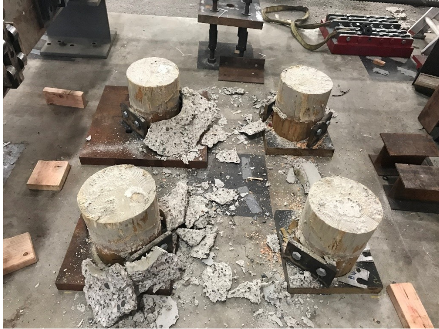
Figure 4.24: Specimen R-S-R-LTi-90-Pile: Damage around piles on pile footing
