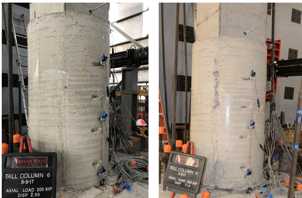
Figure 4.36: Specimen R-T-R-0: Damage progression: (a) at 2.59 in (approx. 1.8%) drift level, (b) at the end of testing (approx. 7% drift level)
