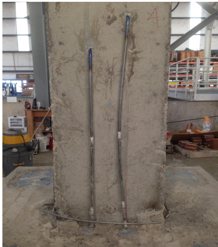
Figure 4.33: RN-T-R-LTi-90: Buckled deformation to WS TiAB ligament (shell removed after testing)
