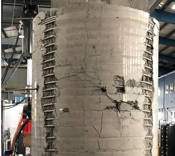
Figure 4.4: Specimen R-S-R-LTi-90: Distress in shell near the TiAB hooks (South face) at the end of testing
