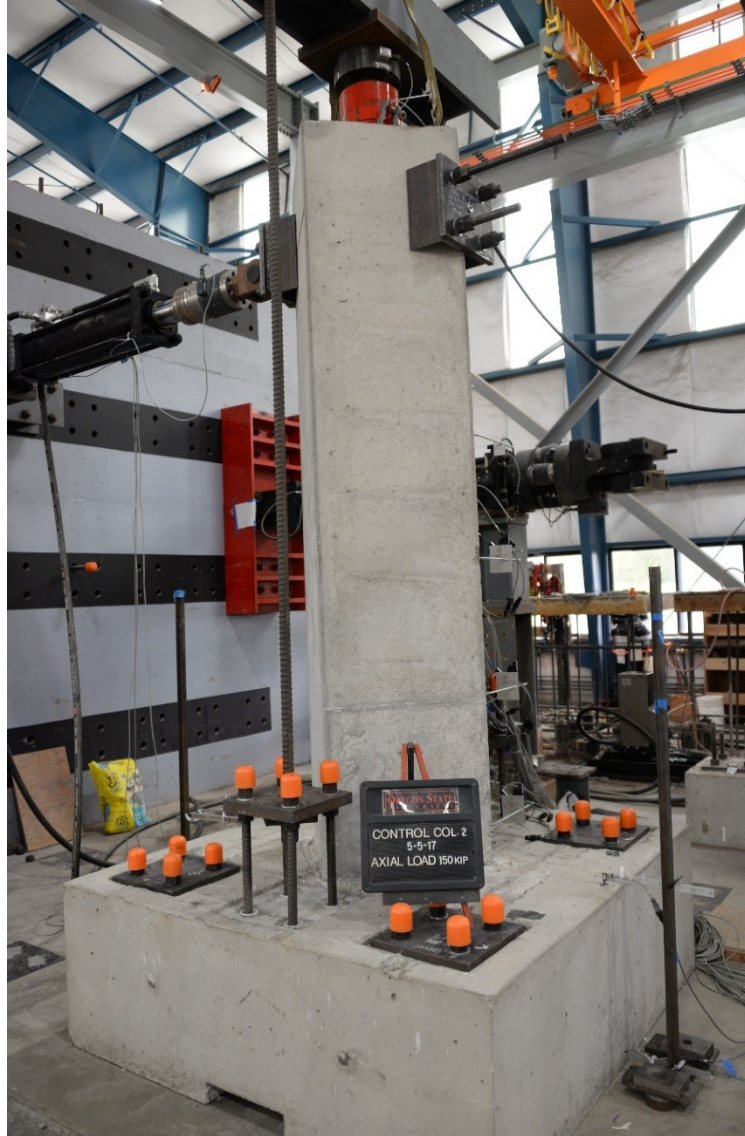
Figure 3.67: Photograph of experimental setup (diagonal control specimen shown with top loading fixture)
