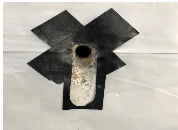
Figure 3.36: Drilled holes for vertical TiAB hook anchorages with rounding at bottom
