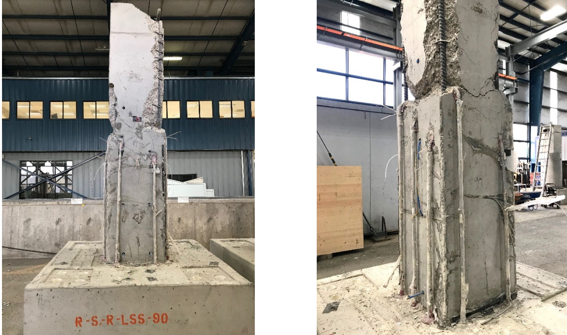
Figure 4.18: Specimen R-S-R-LSS-90: Column after removal of shell: a) Overall, b) Close-up view
