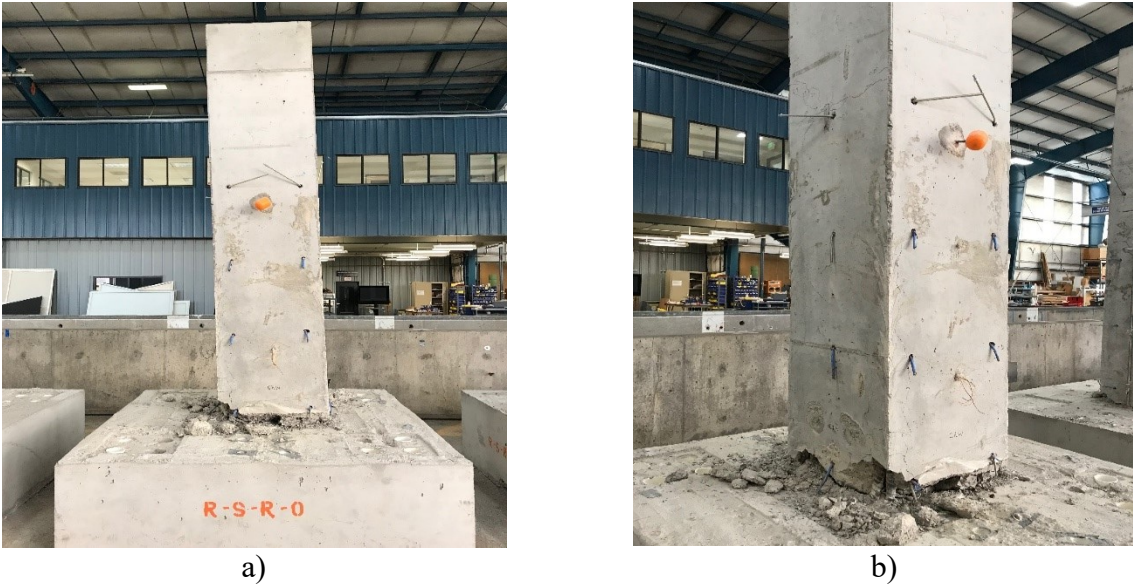
Figure 4.15: Specimen R-S-R-0: Column after removal of shell: a) Overall, b) Close-up view
