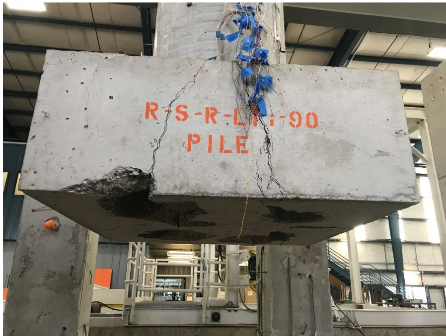
Figure 4.25: Specimen R-S-R-LTi-90-Pile: Cracking on pile cap
