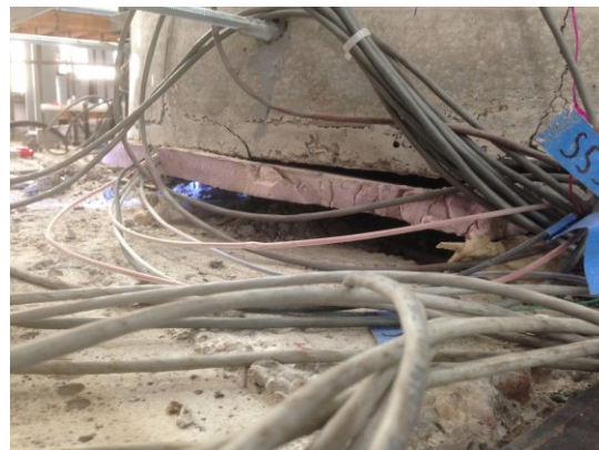
Figure 4.30: Specimen RS-T-R-LTi-90: Foam insulation and opening of shell at top of footing
