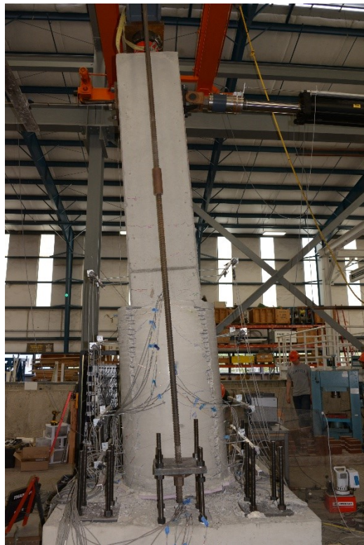
Figure 4.35: Condition of specimen RN-T-R-LTi-90 at end of test (maximum 7.8% drift)
