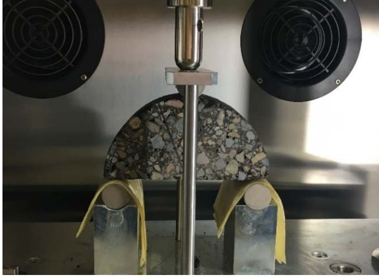
Figure 3.6. SCB loading set up and test
