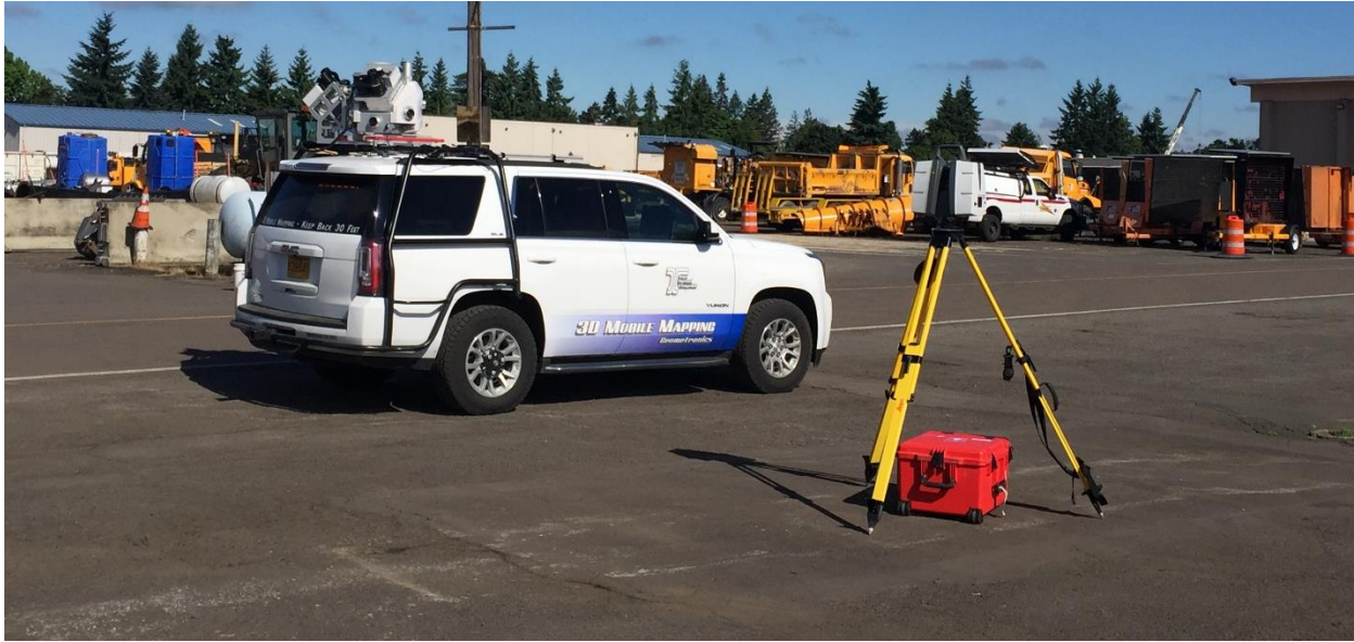
Figure 4.3: Mobile lidar truck with Leica Pegasus: Two and tripod-mounted Leica ScanStation P40 in the foreground.
