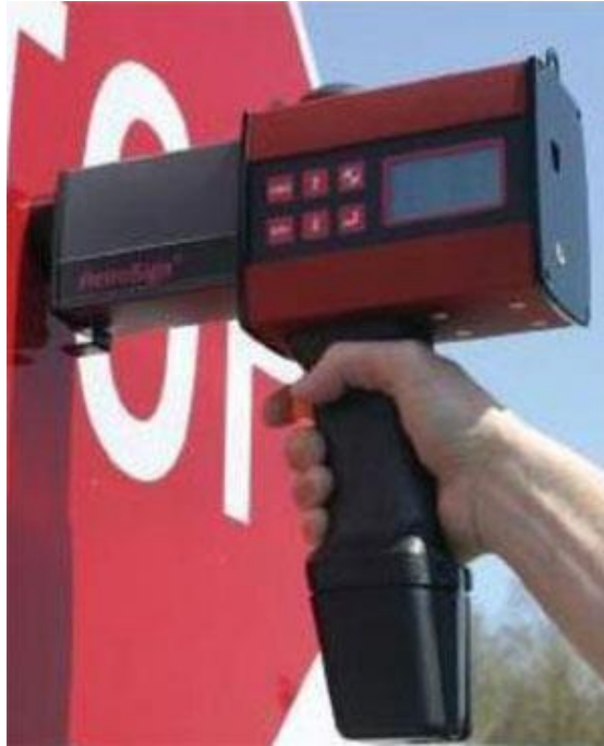
Figure 2.2: Retroreflectometer being used to measure retroreflectance of a stop sign (Figure from FHWA: https://safety.fhwa.dot.gov/local_rural/training/fhwasa09025/fhwasa09025.pdf ).
