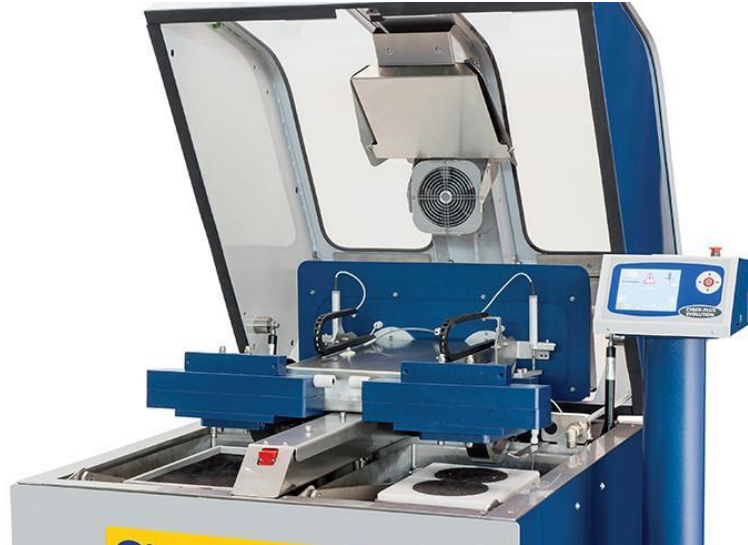
Figure 2.19: Hamburg wheel Tracking Device (Instron-SmarTracker)
