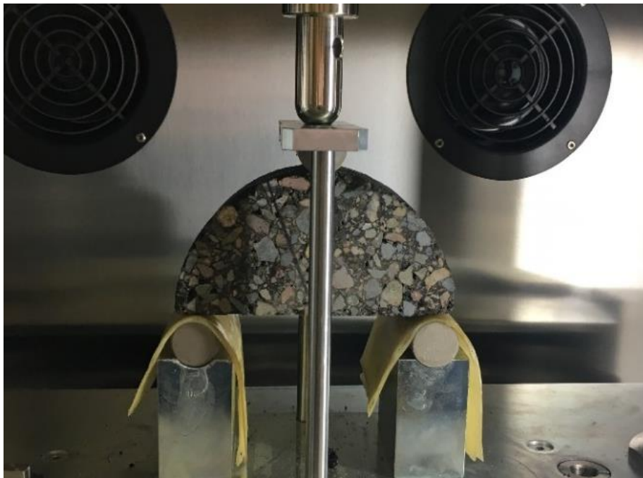
Figure 2.16: SCB loading set up and test
