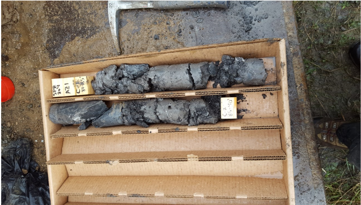
Figure 2.11: Example borehole cores recovered from Arizona Inn during drilling on February 2, 2017. Photograph Credit: Dr Michael Bunn.
