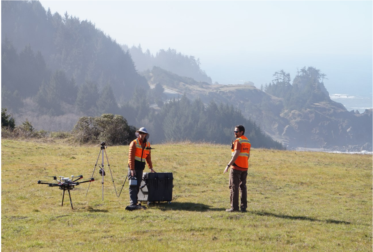
Figure 2.8: Photograph capturing the RAPID Facility’s phoenix lidar miniRanger UAS lidar system being operated at the Hooskanaden landslide on March 15, 2019. Photo Credit: Nick Mathews (OSU).
