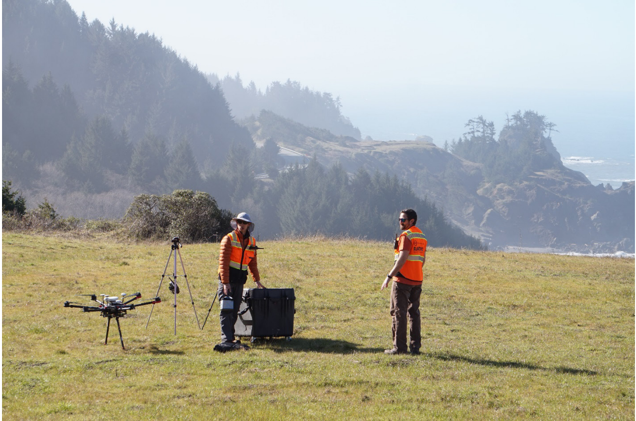
Figure 4.9: Photograph capturing the RAPID Facility’s phoenix lidar miniRanger UAS lidar system being operated at the Hooskanaden landslide on March 15, 2019. Photo Credit: Nick Mathews (OSU).
