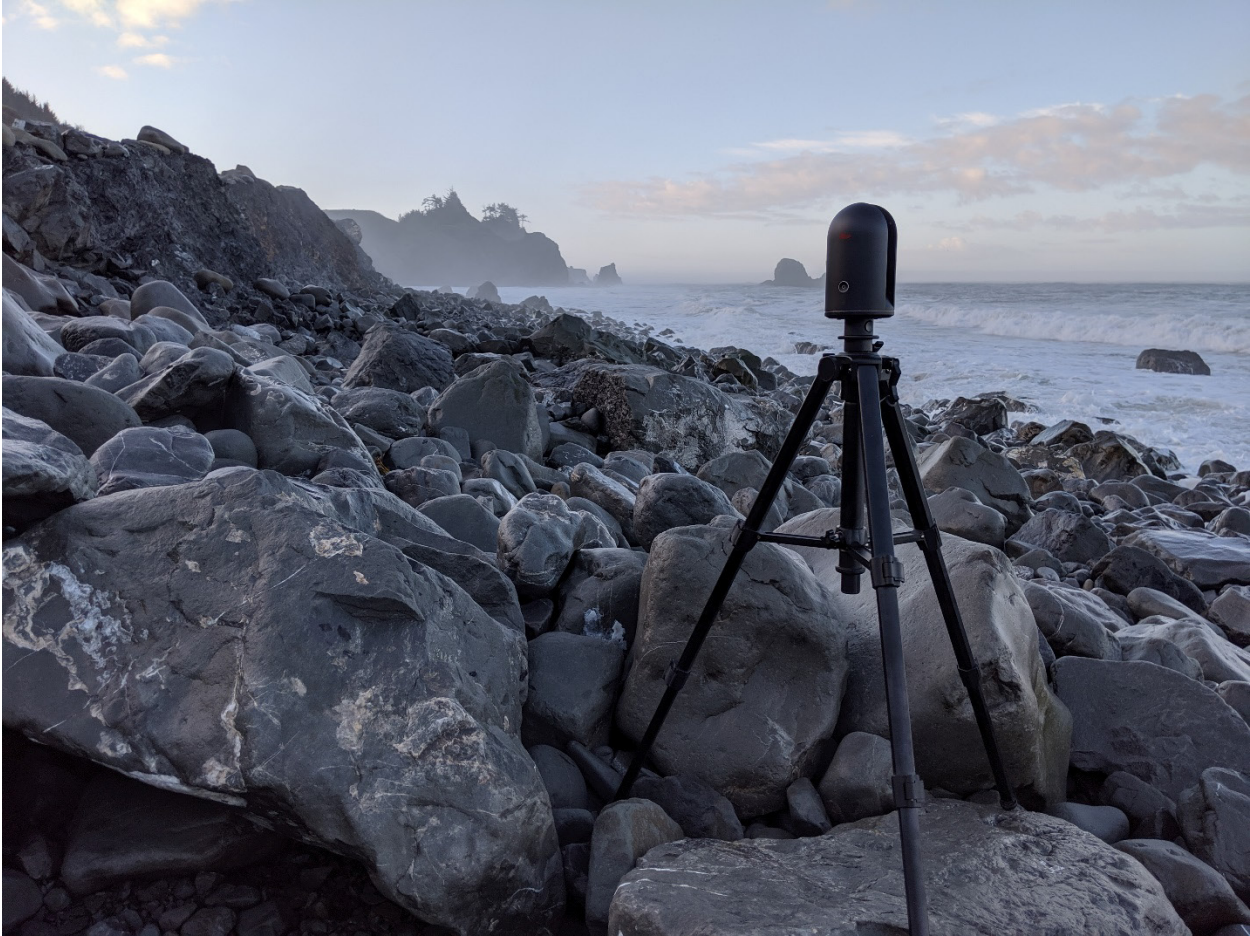
Figure 4.7: Photograph of the BLK360 TLS (terrestrial laser scanner) being used to survey the sea cliff at the Hooskanaden beach during the bi-annual field survey on October 4, 2019.
