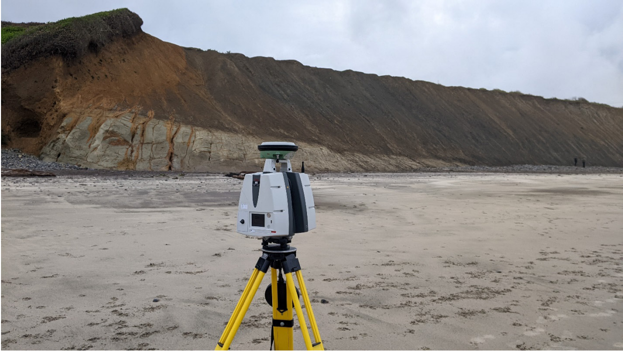
Figure 4.1: Example terrestrial laser scan setup with GNSS sensor for georeferencing.
