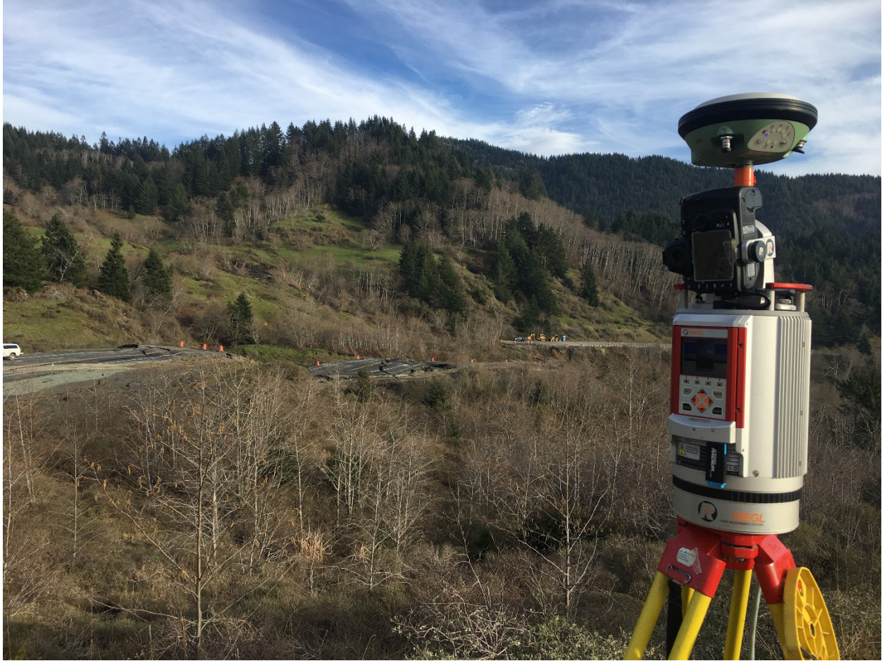
Figure 4.8: Photograph of Riegl VZ-400 TLS setup to conduct high resolution repeat scans of the actively moving Hooskanaden landslide on March 2, 2019.
