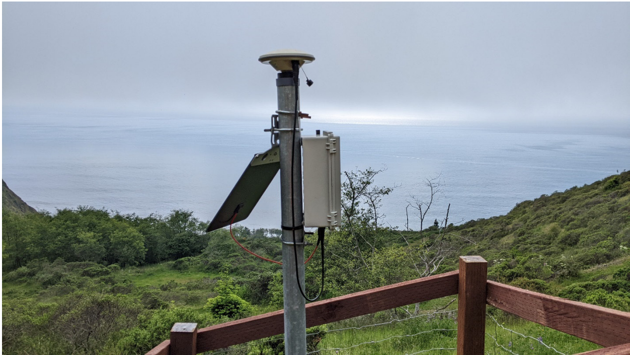
Figure 8.5. Example RTK GNSS rover system installed at the Arizona Inn site.
