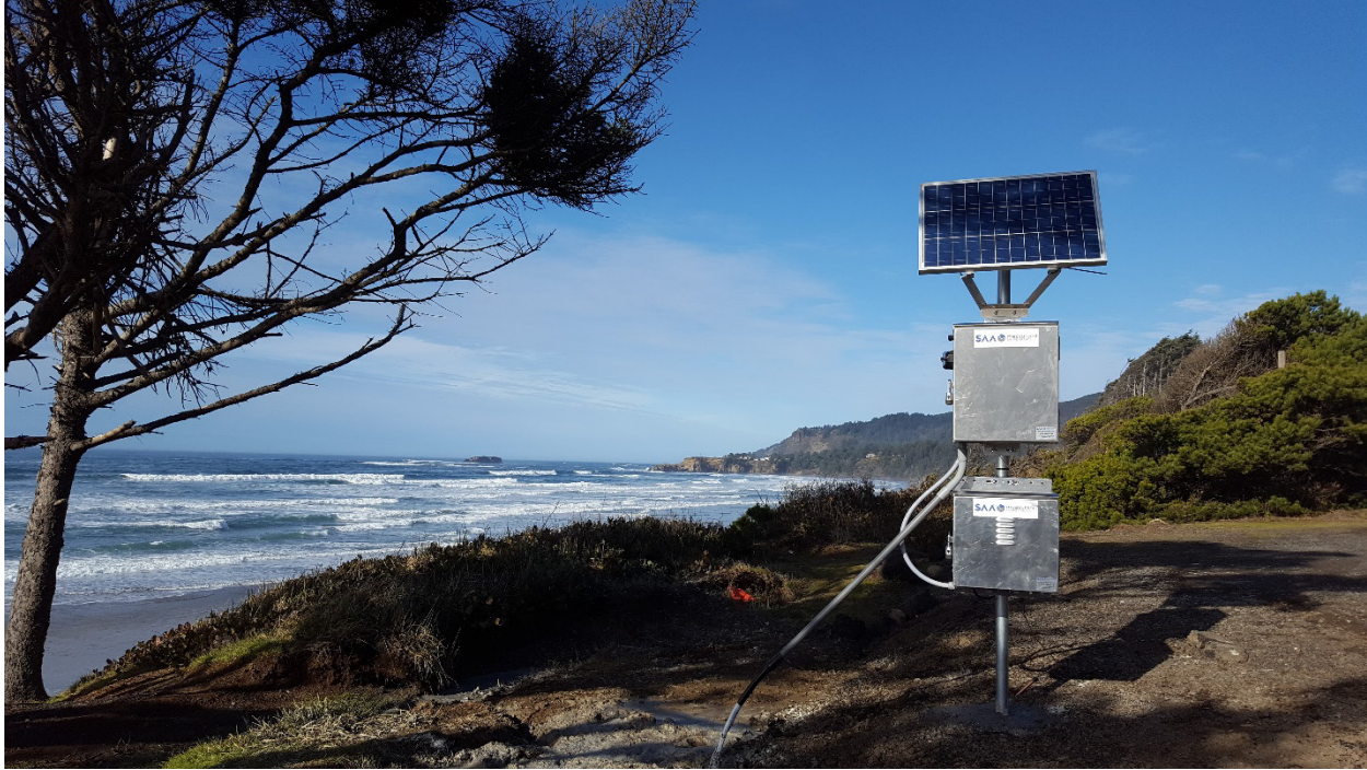
Figure 8.4: Final SAA MEM’s sensor setup at Spencer Creek on January 27, 2017. Composed of solar panel for power supply, SAA electrical components (top box), SAA battery (bottom box), and SAA sensor (in borehole). Photograph Credit: Dr Michael Bunn.
