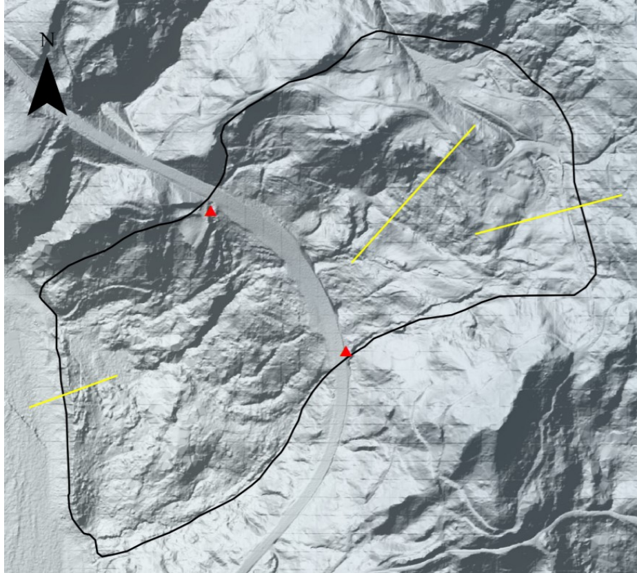
Figure 4.5: Locations of TLS data collection (red triangles), and field developed cross-sections (yellow lines), overlying 2015 lidar and hillshade derivative.
