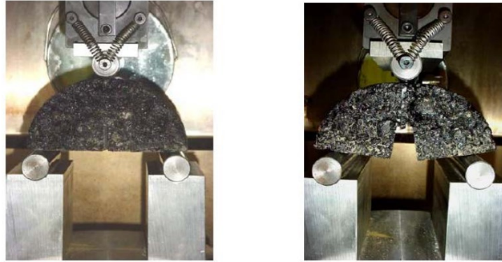
Figure 2.13: Semi-circular bend (SCB) test apparatus (Wu et al. 2005)
