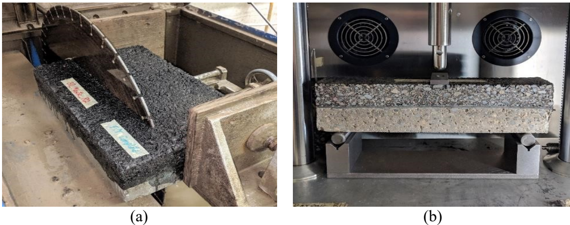
Figure 5.16: Three-point bending sample preparation and testing (a) Cutting of three-point bending sample (b) Three-point bending sample positioned in UTM
