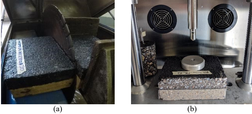
Figure 5.14: FN sample preparation and testing (a) Cutting of FN samples (b) FN sample positioned in UTM
