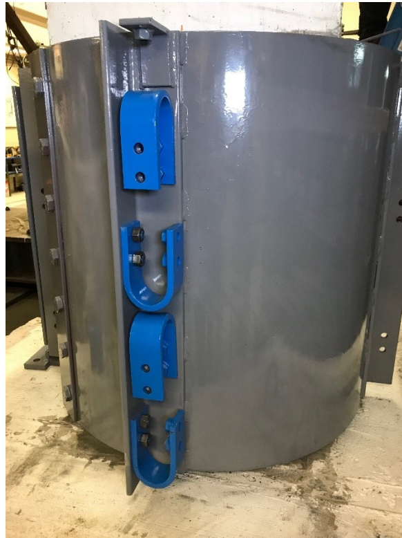
Figure 4.4: UFPs inside hold-down
