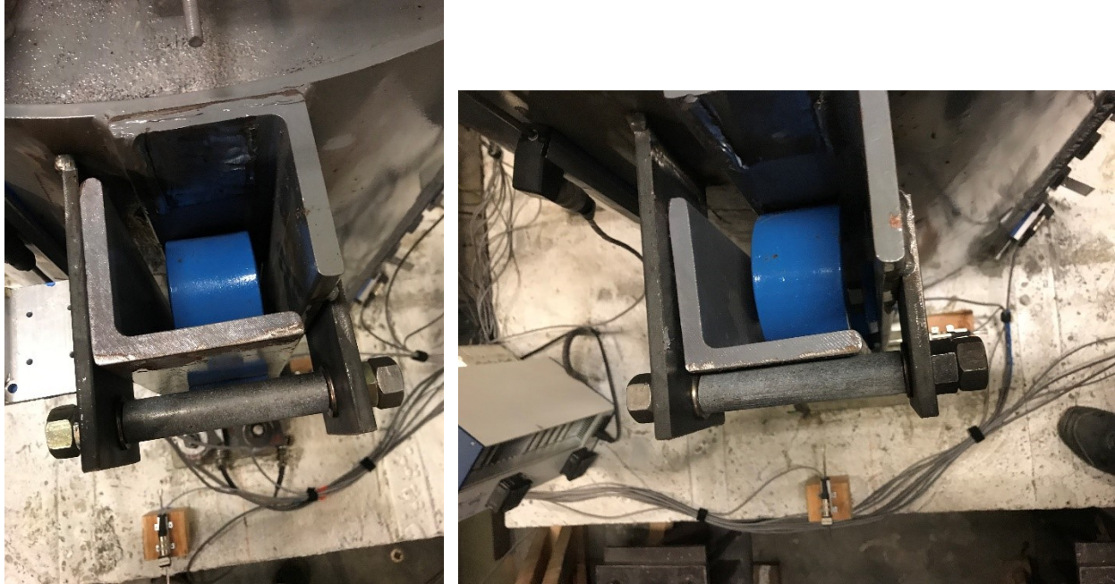
Figure 5.10: Hold-down rollers (a) before and (b) after test
