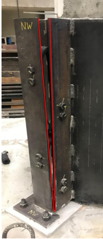
Figure 5.3: Residual hold-down deformation
