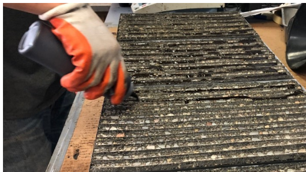
Figure 4.6: Application of tack coat using condiment bottle for coverage/streaking samples.
