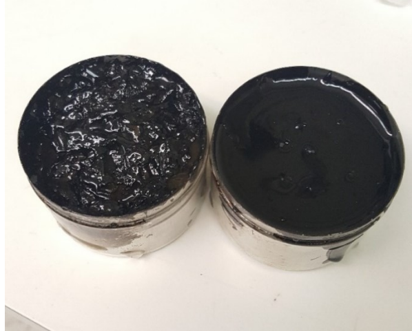
Figure 3.15: Comparison of CO2-ENGR-M binder (left) and CO1-CSS1H binder (right)
