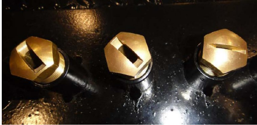
Figure 2.33: Various nozzle sizes corresponding to different application rates (FHWA 2016).
