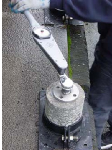
Figure 2.25: Torque bond test device (Tashman et al. 2006).
