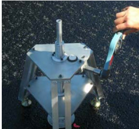
Figure 2.23: Texas pull-off test (Tashman et al. 2006).
