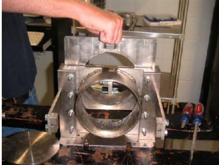
Figure 2.16: Florida direct shear test device (Tashman et al. 2006).
