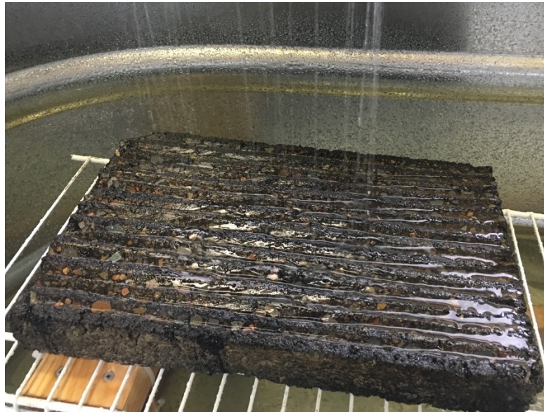
Figure 4.7: First lift samples in the rainfall simulator.
