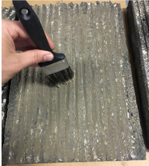
Figure 4.5: Dust being applied to pavement surface.
