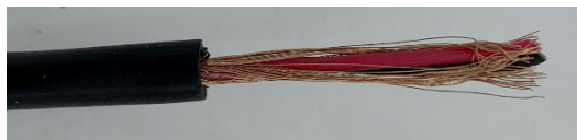
Figure 7.12 Transducer cable with outer jacket stripped back.
