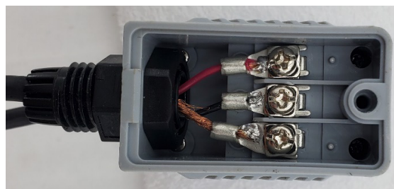
Figure 7.16 Wires with fork spades attached inside transducer head. Note the cable gland nut is not shown but should already be on the cable in orientation shown in Figure 21 (top).
