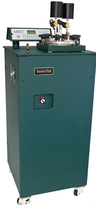
Figure 4.3: Moisture-induced sensitivity tester (MIST) equipment (InstroTek 2011)
