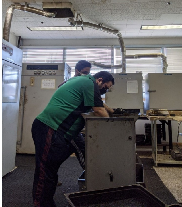
Figure 4.1: Mechanical splitting of asphalt mixtures
