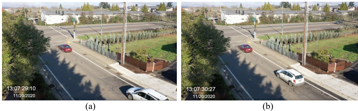
Figure 3.7: Detector 19 on the NB approach of US20 and 15th Street. (a) Detector 19 call on. (b) Detector 19 call off.
