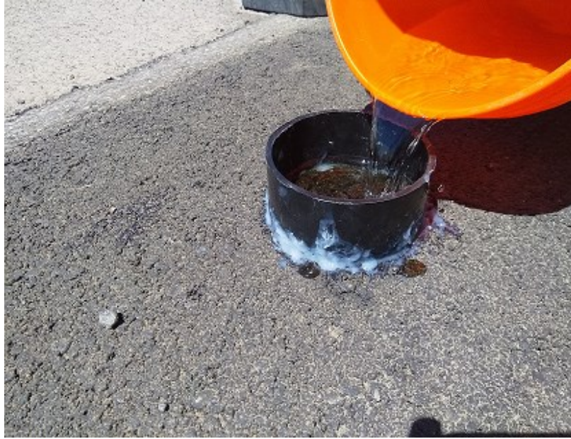
Figure 4.4: Field infiltration test
