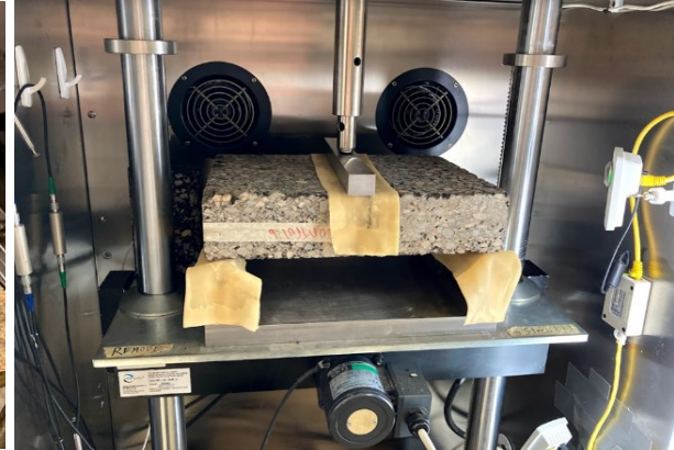
(b) Three-point bending sample positioned in the Universal Testing Machine (UTM)
