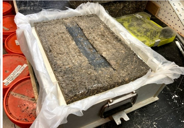
(b) Tested CLRS block sample with cracking
