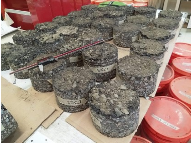
(g) Sampled asphalt cores
