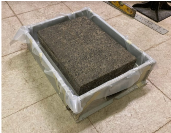
(c) Asphalt sample centered in HWTT mold
