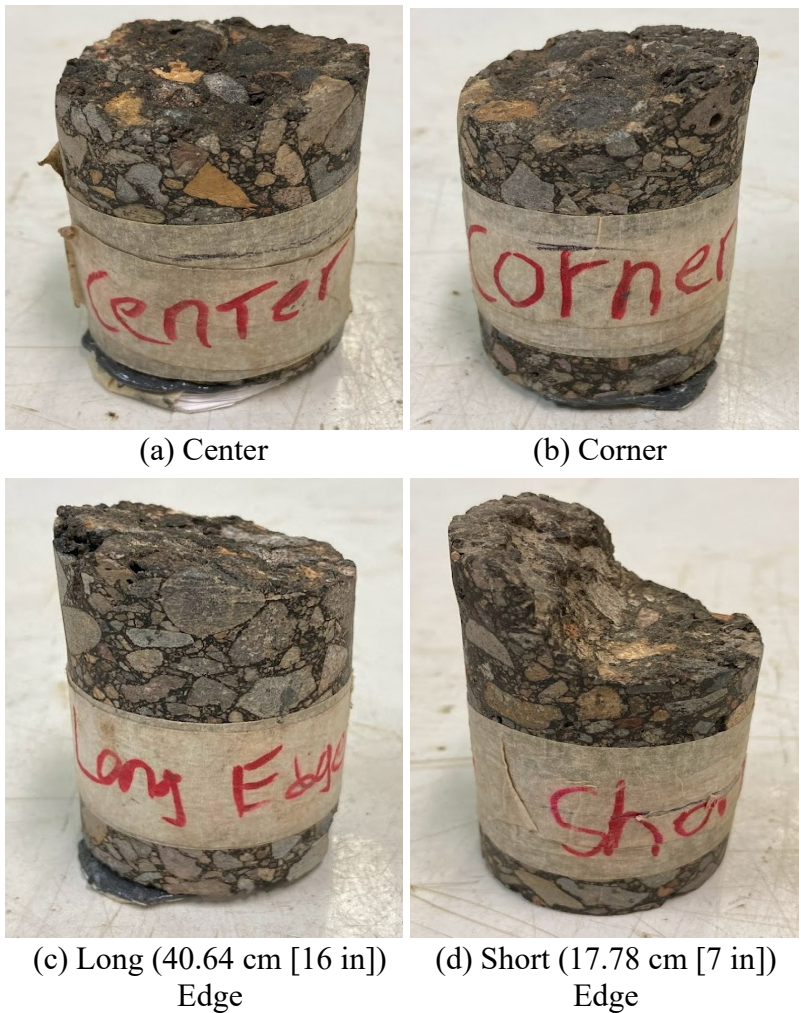
Figure 4.20: Cores for X-ray CT imaging
