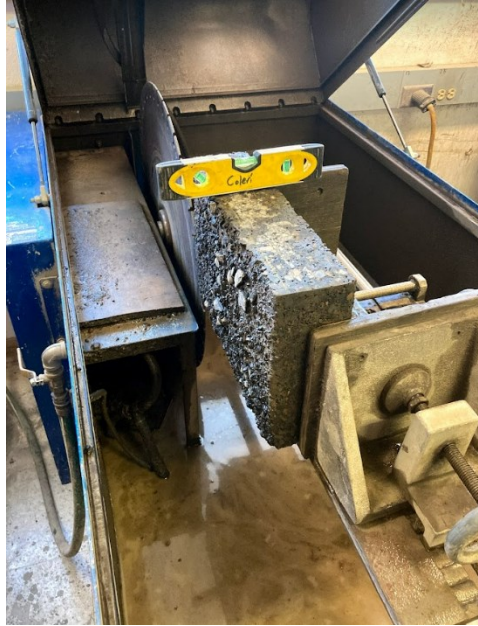
Figure 4.8: Cutting samples using water-cooled diamond blade
