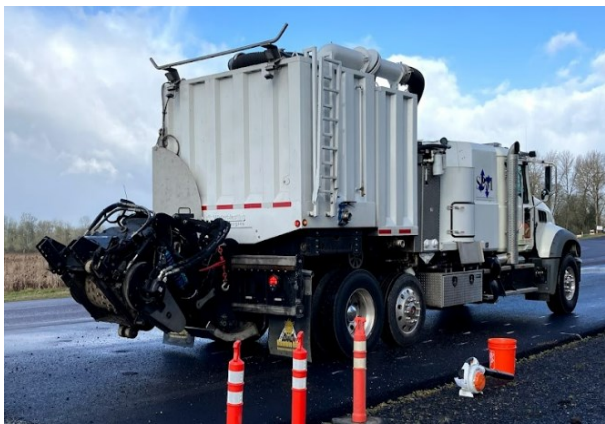
(d) Milling equipment (courtesy Specialized Pavement Marking, Inc.)
