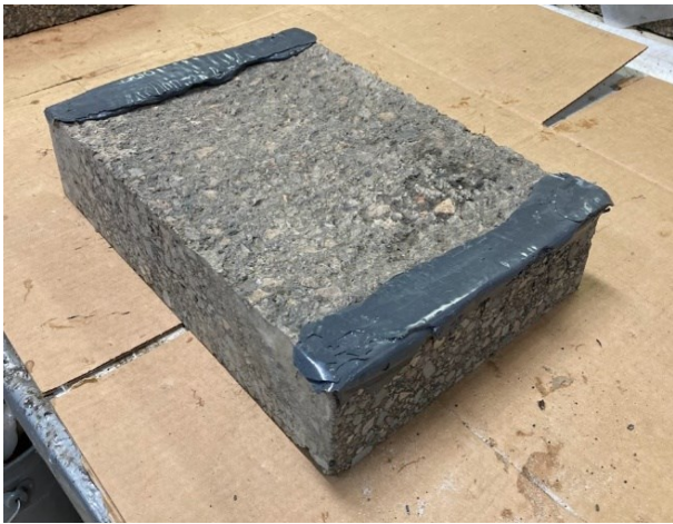
(c) Devcon used to flatten ends due to rumble strip curvature
