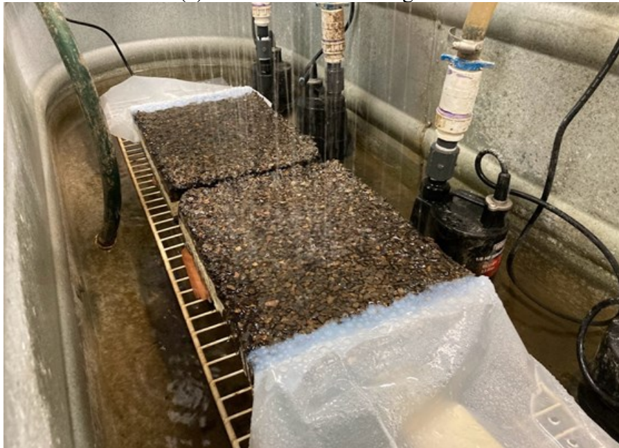
(b) Sample undergoing infiltration test
