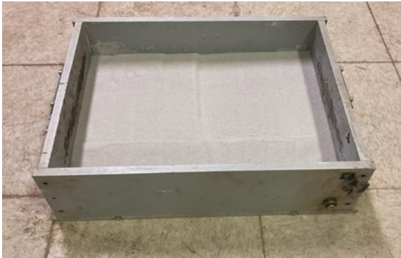
(a) HWTT mold with sand base layer
