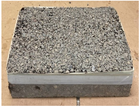
(f) Finished CLRS chip seal block sample
