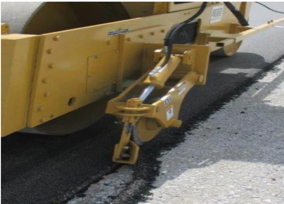
Figure 2.13: Roller mounted with a cutting wheel. ( https://www.equipmentworld.com )
