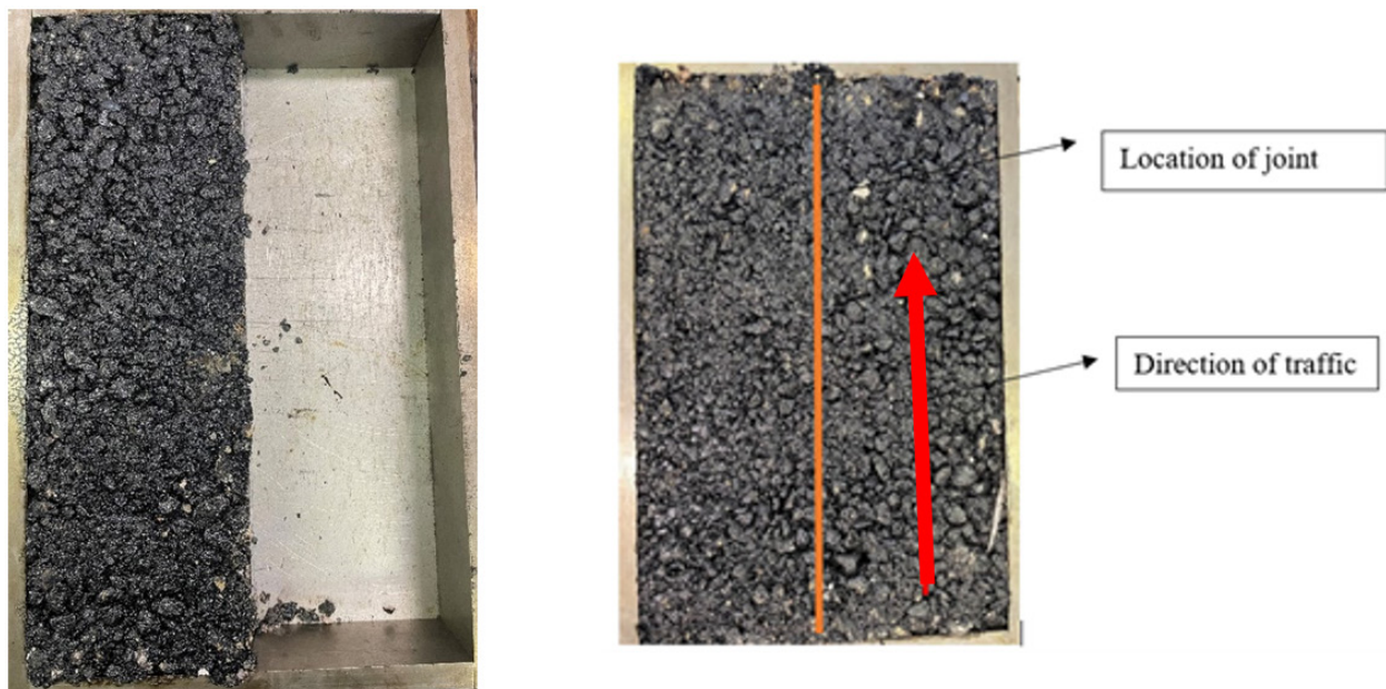
Figure 4.4: Sample preparation for restrained edge longitudinal joint construction: a) Half specimen after compaction and removal of steel spacer, b) Final specimen.
