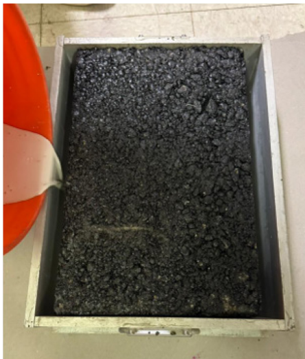
d) Plaster applied on the sides
