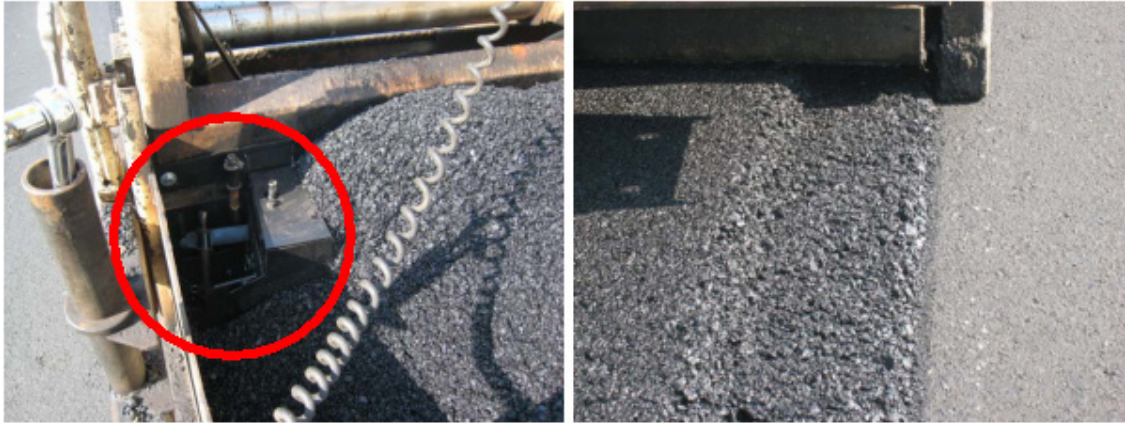
Figure 2.25: Notched Wedge Joint Maker by TransTech Systems, Inc. (Williams 2011)
