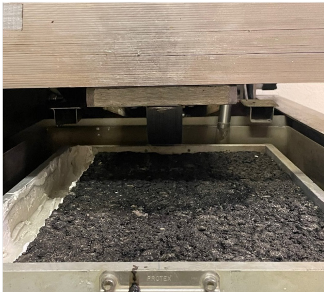
a) Placement of the longitudinal joint sample in the test equipment
