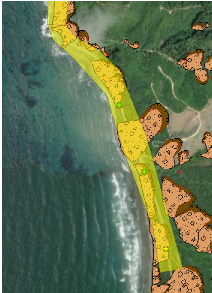
Figure 3.3: Example site with multiple unstable slopes within the zone that were aggregated to extract different hazard parameters.
