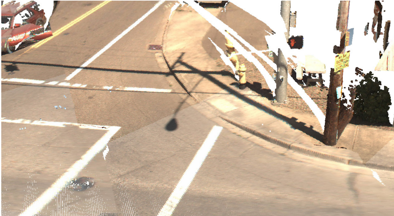
Figure 2.8: Example of pointcloud data at a curb ramp collected by Leica Pegasus: Two mobile lidar system.
