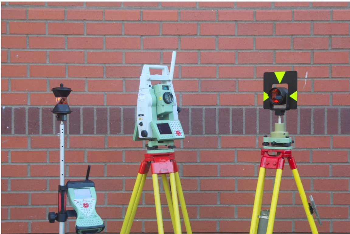
Figure 2.5: Total station, remote controller, and prism.
