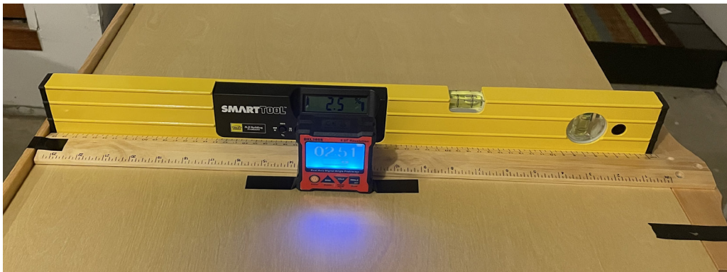
Figure 3.3: Example setup with a smart level and smaller digital inclinometer.
