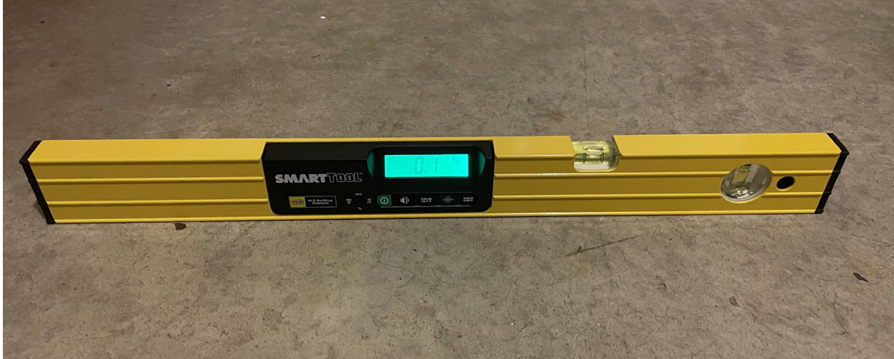
Figure 2.3: Example SmartTool ® digital inclinometer (2-ft or 60-cm length).
