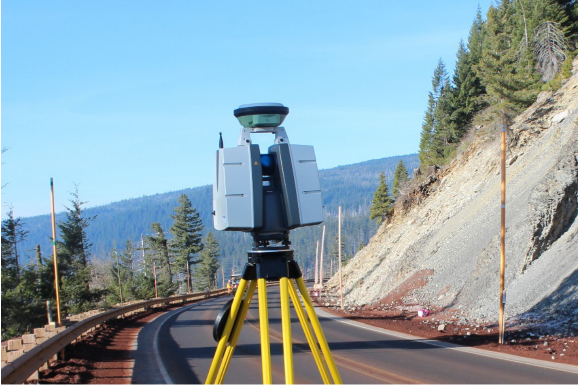
(b) A survey-grade Leica ScanStation P40 scanner
