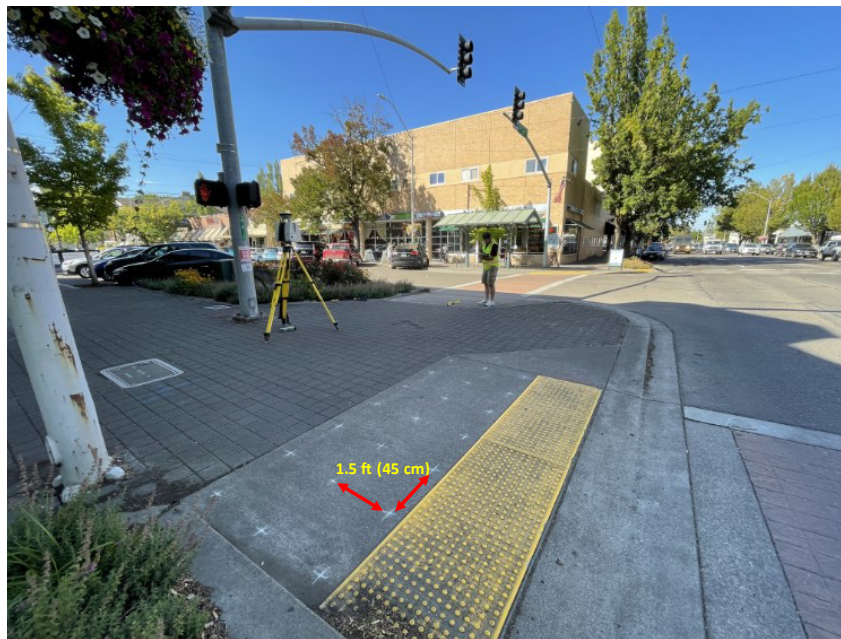
Figure 7.3: Example sampling grid marked with chalk for slope measurements.
