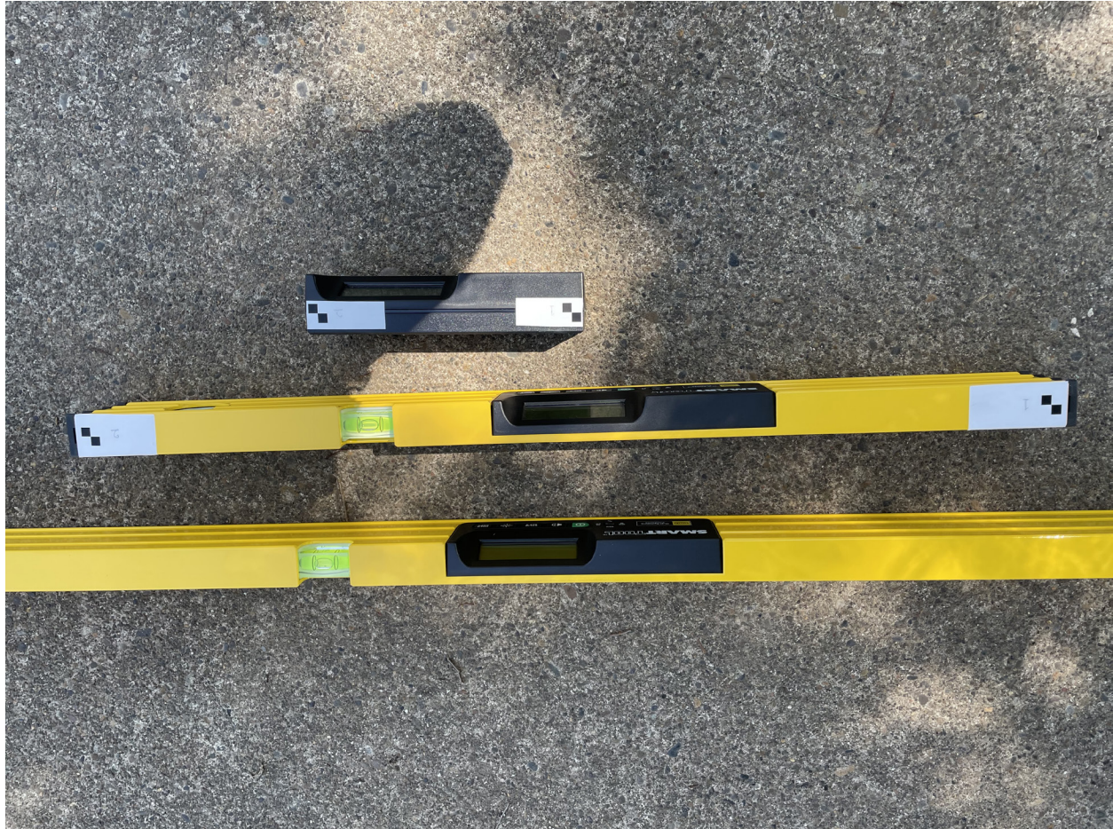
Figure 5.2: Smart levels used in the operator variability test with end points marked.
