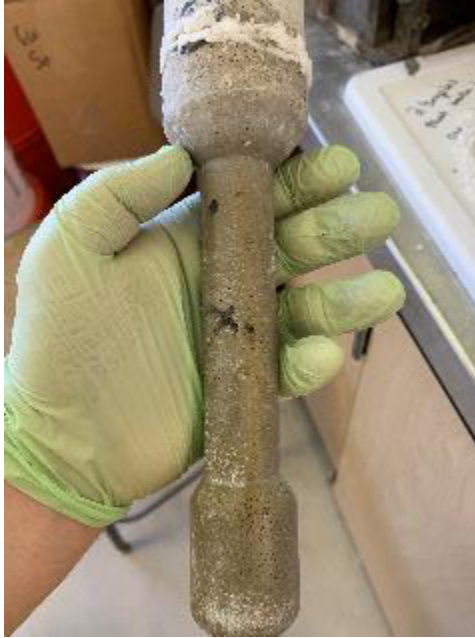
Figure 4-28. Corrosion precipitate and staining on PrCSA2 sample
