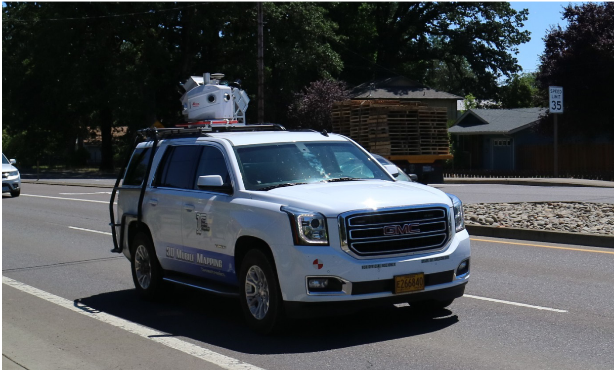
Figure 2-15: Oregon DOT's current mobile lidar system, Leica Pegasus:Two
