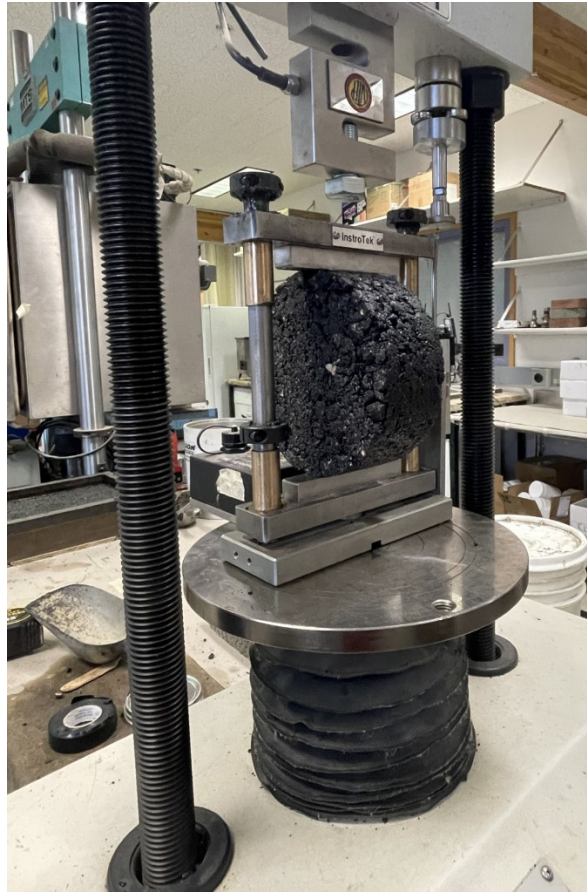
Figure 4.3: IDT-CT test setup.
