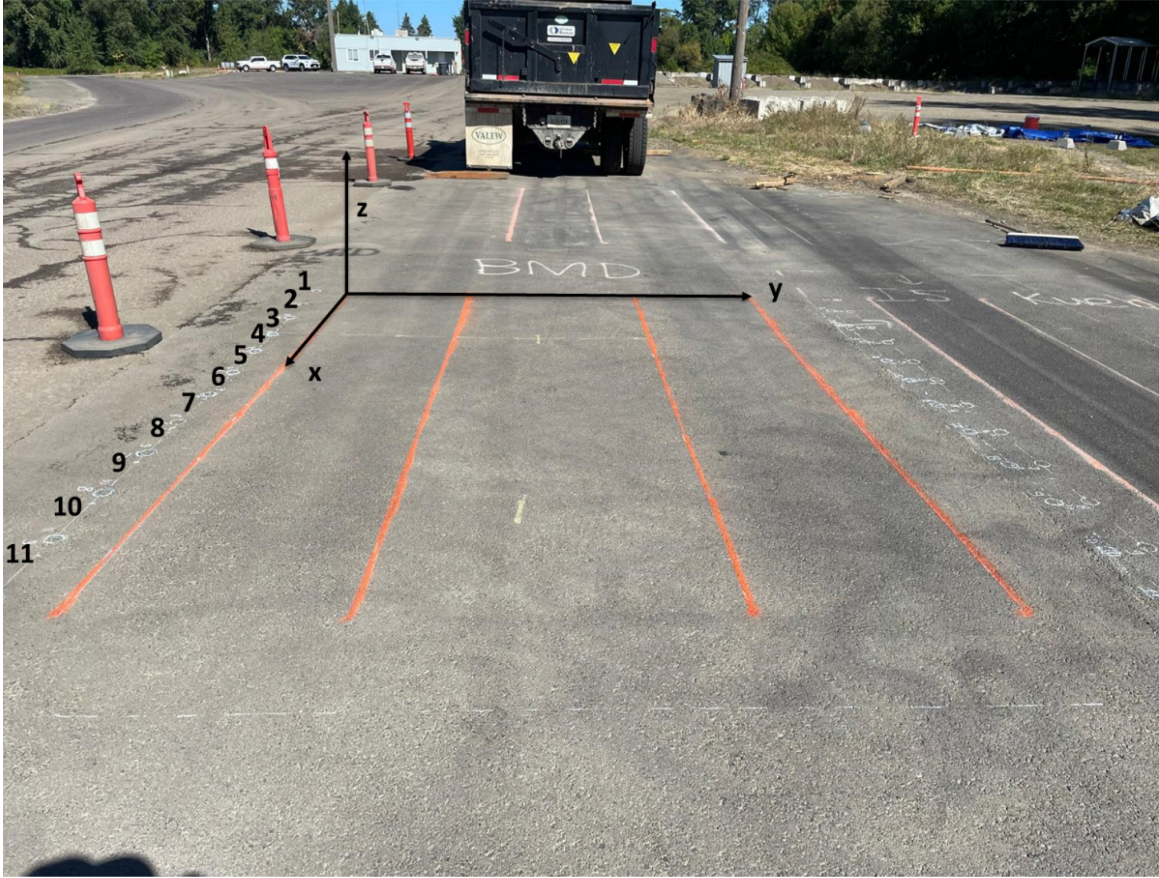
Figure 6.6: Profilometer measuring stations marked on the BMD section and coordinates used in this study.
