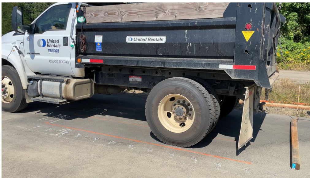
Figure 6.4: Marked the Volumetric section and loading the section with the dump truck
