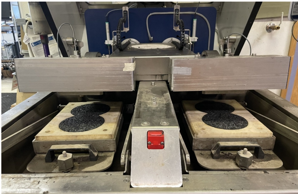
Figure 4.2: HWTT set up.
