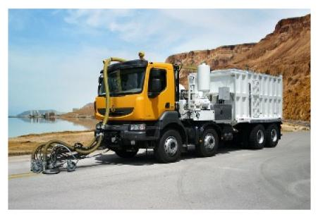
FIGURE 2.2: HIGH-PRESSURE WATER BLASTING TRUCK (GOOGLE, 2021)
