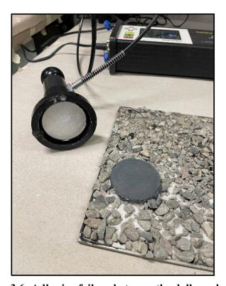
Figure 3.6: Adhesive failure between the dolly and epoxy
