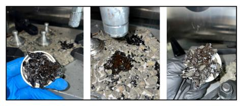
Figure 3.16: Samples after the pull-off tests (5°C) (brown color showed insufficient curing)
