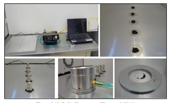
Figure 2.10: Pull-off test setup (Zhou et al. 2014)
