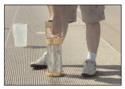
Figure 2.21: Outflow test meter application in the field (Aktas et al. 2011)
