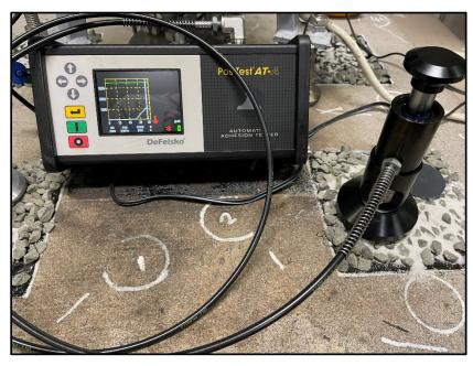
Figure 3.5: Trial tests with PosiTest on chip seal samples
