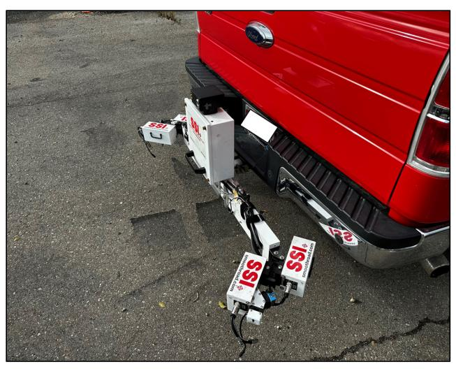
Figure 5.5: High-speed profiler system used in this study (Photo credit: Alejandro Rosales of Idaho Asphalt)
