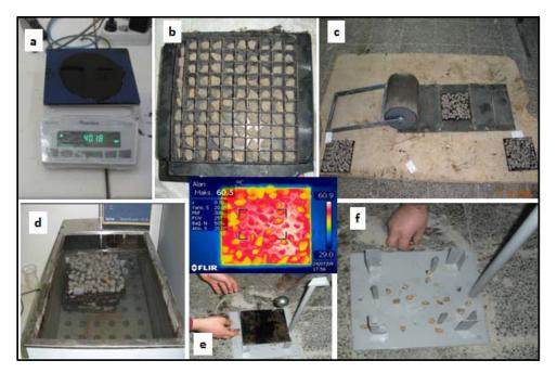
Figure 2.6: Vialit test described in EN 12272-3 (a) emulsion-asphalt cement application; (b) spreading chips; (c) compaction; (d) curing of chip seal samples; (e) free fall of the ball over the plate; (f) counting fallen chips (Gurer 2010)
