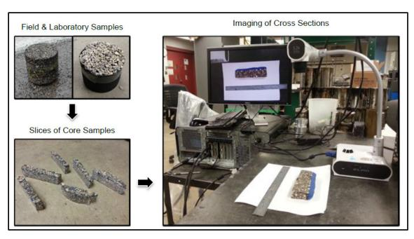
Figure 2.23: Stages of determination of percent embedment (Kutay et al. 2016)
