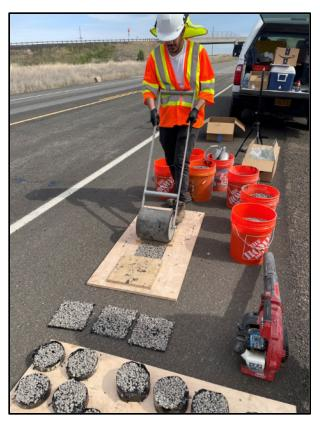
Figure 3.20: Compacting samples after emulsion and aggregate application
