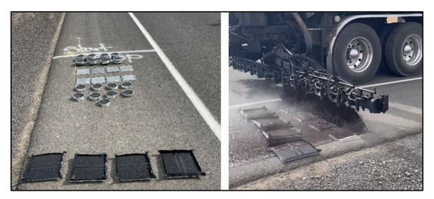
Figure 4.2: OreTackRate system for measuring EAR of chip seal
