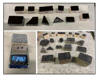
Figure 3.11: Steps for calibration of effective binder area measurement
