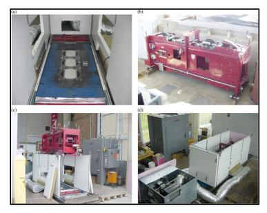
Figure 2.24: MMLS3 test setup: (a) mounting of samples on steel platform (b) MMLS3 device (c) placing the device in a climate chamber (d) MMLS3 test ready to perform a test (Adams and Kim 2014)
