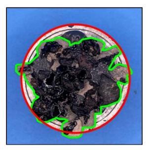
Figure 3.10: Pull-off test dolly after the test. The red circle shows the area for the circular method, while the green lines show the Pline method
