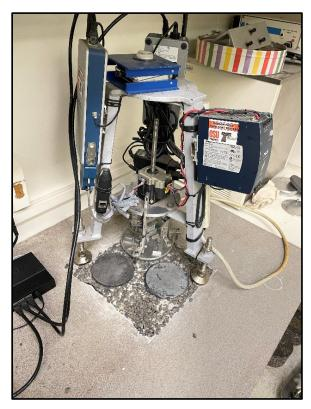
Figure 3.4: Trial tests with the OFTCT on chip seal samples
