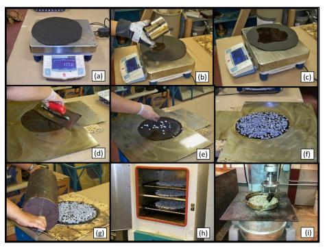
Figure 2.7: Sweep test (ASTM D7000 2019) conducted on chip seal sample (a) preparation of asphalt felt disc; (b-c) applying emulsion on asphalt felt disc; (d) flatting the emulsion surface; (e-f) chip spread process; (g) compaction of chip seal sample; (h) curing the specimens in the oven; (i) performing sweep test using mixer and nylon brush (Wasiuddin et al. 2013)
