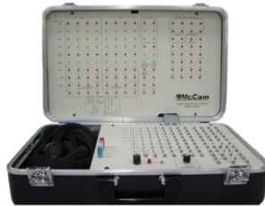
Figure 4. Example of a Controller Tester
