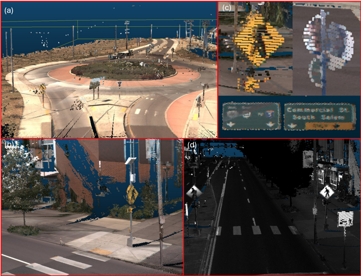
Figure 3.5. Considerations in annotating traffic signs (a) Close proximity to the road ways (b) Close proximity to the crosswalks (c) Different signage shapes (d) High reflectance/intensity of traffic signs.
