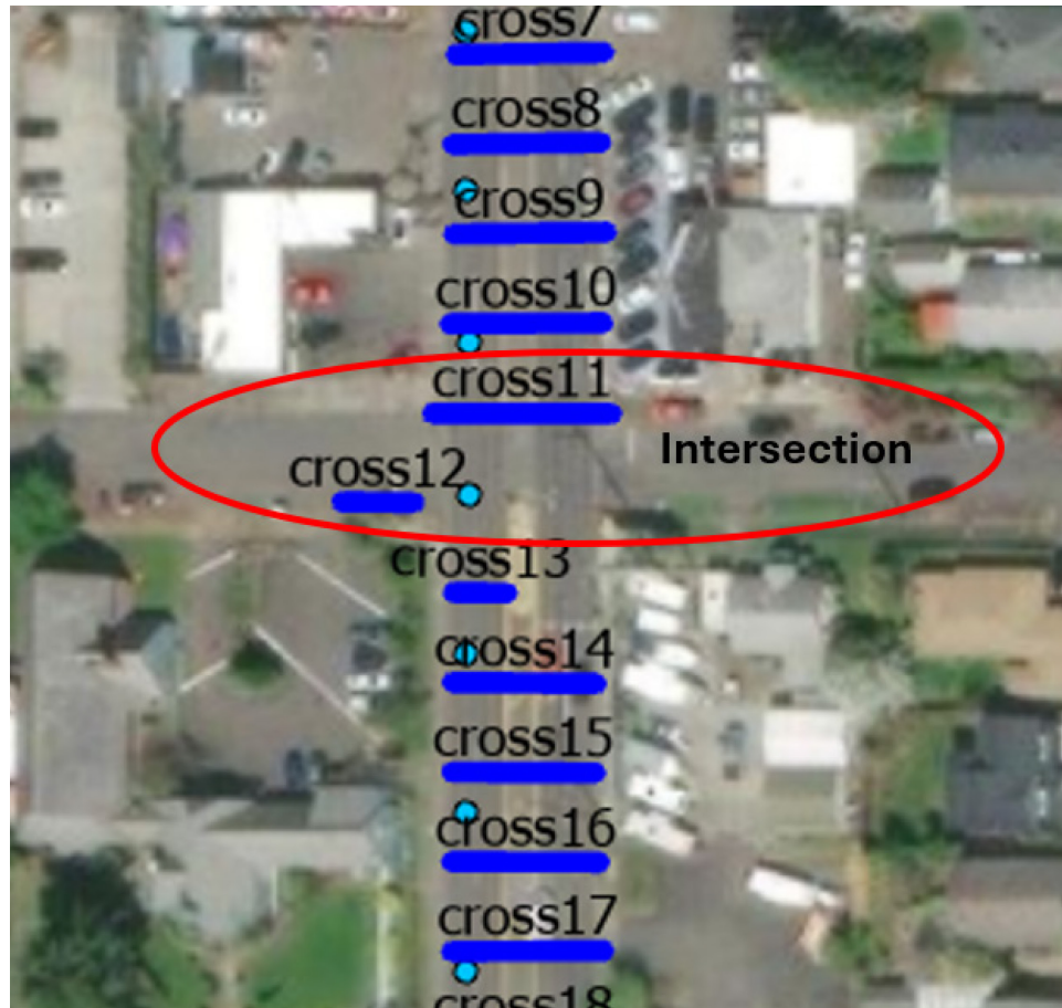
Figure 5.17 Example of incorrectly detected cross sections near an intersection with raised median presence
