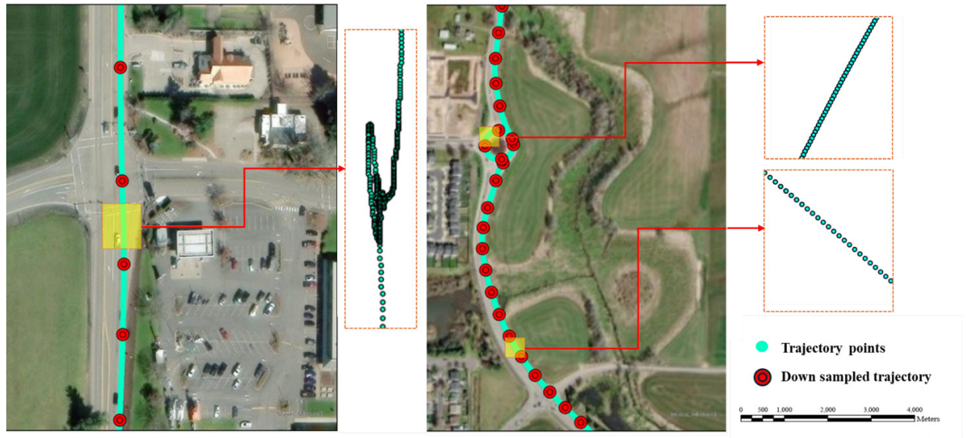
Figure 5.4 Example of variant point spacing and down-sampling results of the mobile lidar trajectory data
