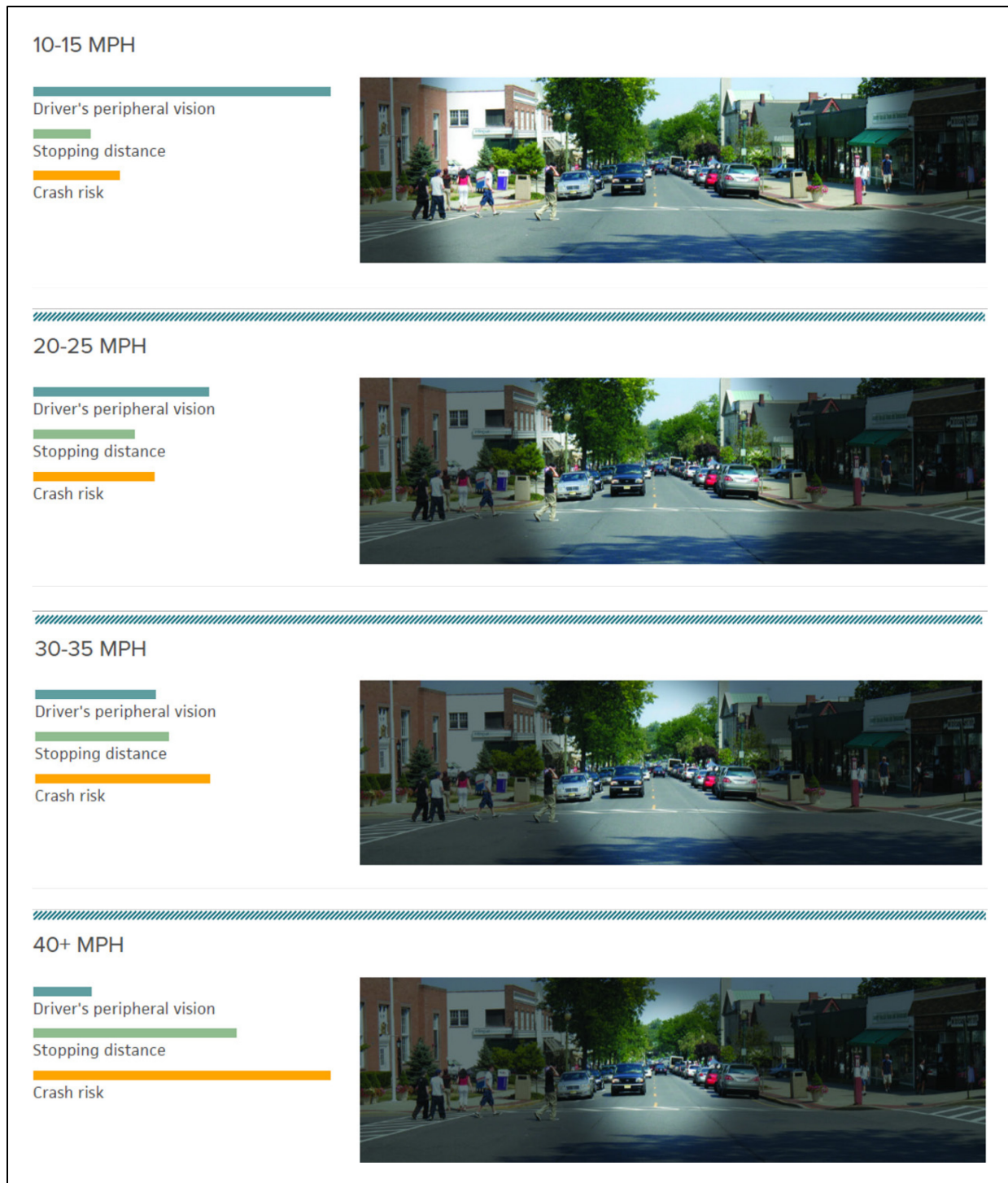
Figure 2.8. Relationship Between Speed & Driver's Peripheral Vision (NACTO, 2013)
