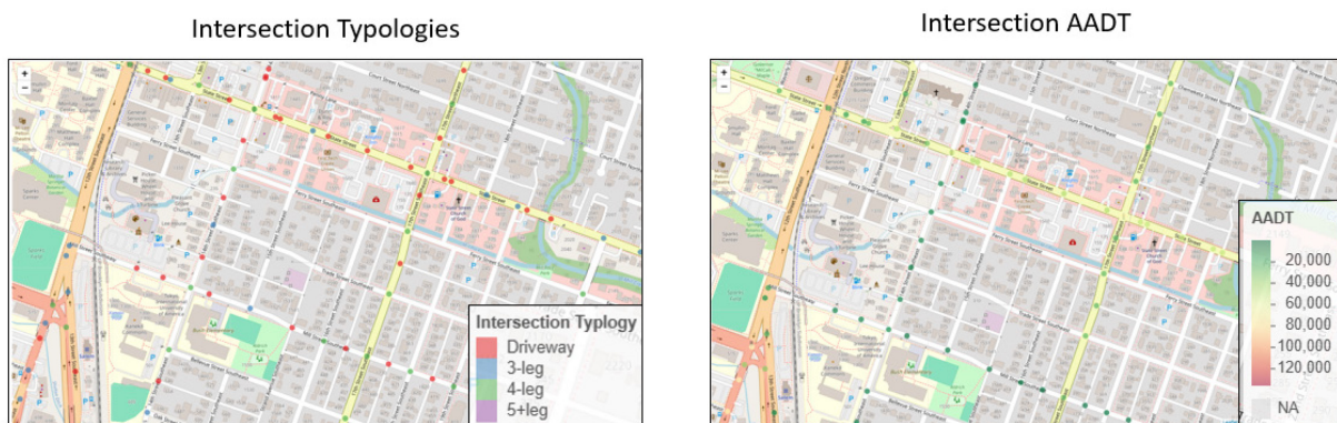
Figure 3.9: Example of Step 4a through Step 4d – Intersection Typology and Entering AADT
