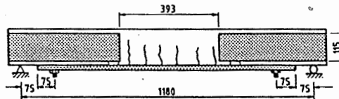
Various repair schemes for damaged beams: (c) Additional plates (wings bonded to beam sides)
