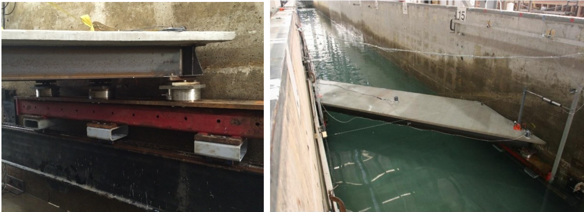
Figure 1.10: Skewed bridge specimen used as a benchmark problem for the validation of the three-dimensional formulation of the CFD solver
