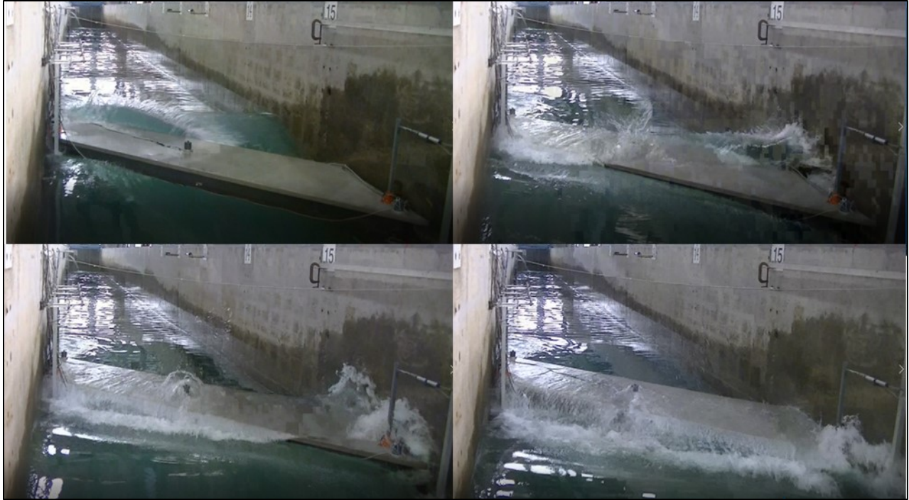
Figure 1.12: Snapshots of the skewed bridge inundation process recorded in the experiments for H=0.55\text{m}
