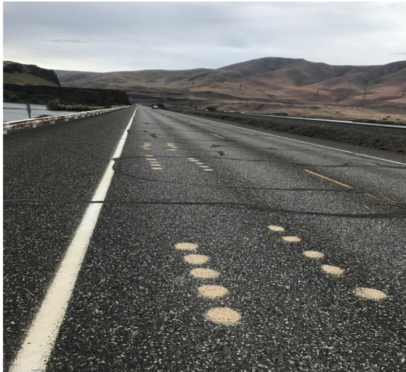
Figure 9.6. Sand circle tests prior to construction
