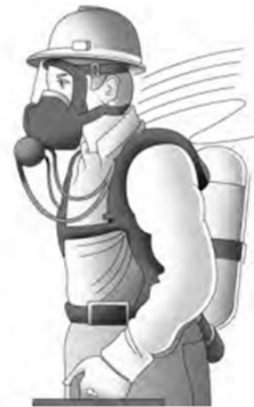
Full Facepiece Self-Contained Breathing Apparatus (SCBA) Pressure demand mode is APF=10,000 Needs to be fit tested
