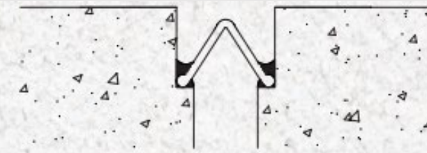
Silicoflex installed in stepped concrete headers
