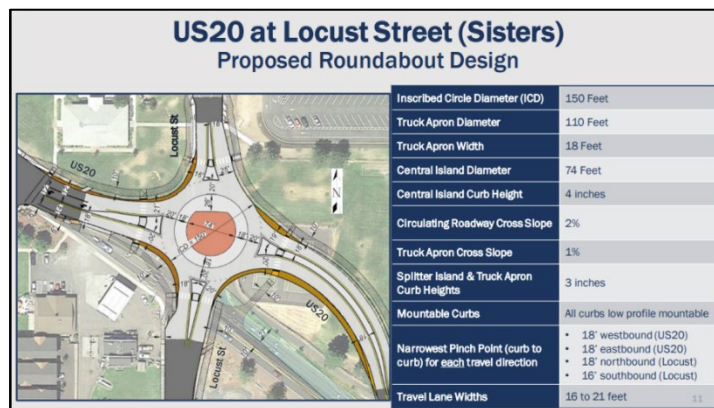
Figure 4: Example of slide showing roundabout design elements.
