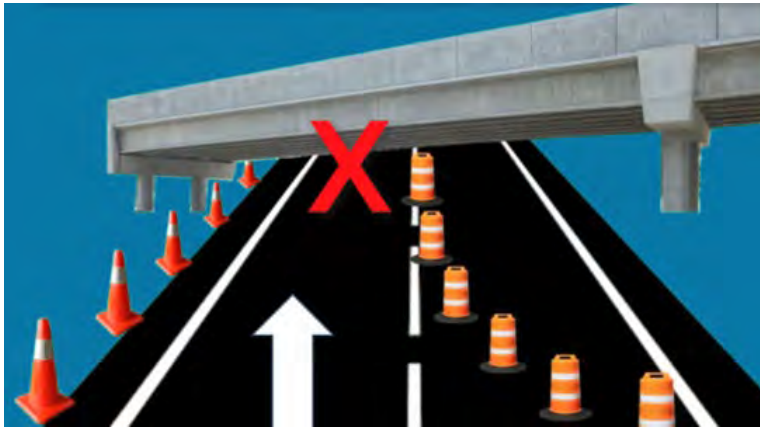
Figure 7: A lane closure/lane shift under a structure can result in lower vertical clearance
