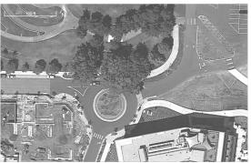
Here is an image of our highway roundabout design compared to the C Street and Osprey Lane roundabout in Independence. The C Street and Osprey Lane roundabout is about half the size of our design for the OR 99W and Clow Corner Road intersection.
