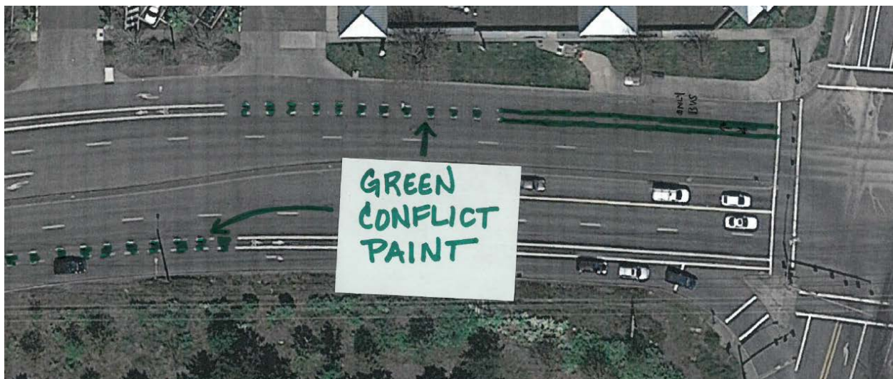
Exhibit 69. Shorten transition into westbound right-turn lane by striping and/or potential curbing
