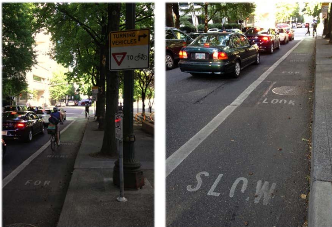
Exhibit 88. Example signage and pavement markings for northbound right-turn
