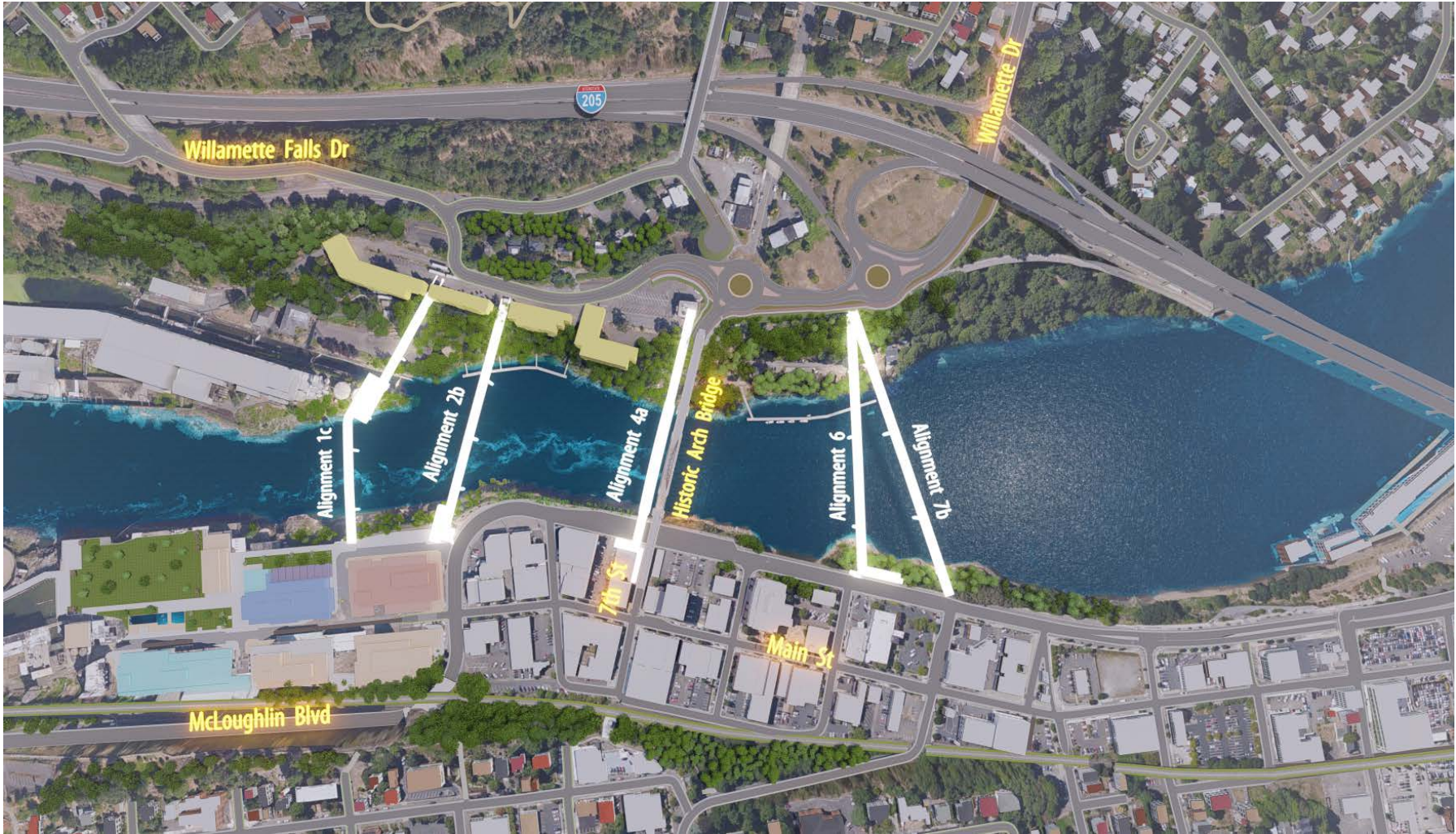
Figure 1: Potential Bridge Alignments
