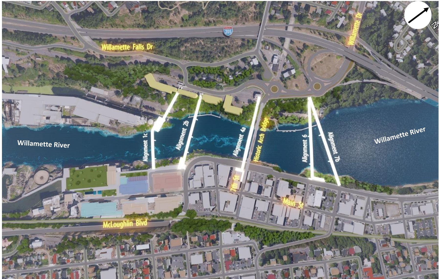
Figure 1: Potential Bridge Alignments
