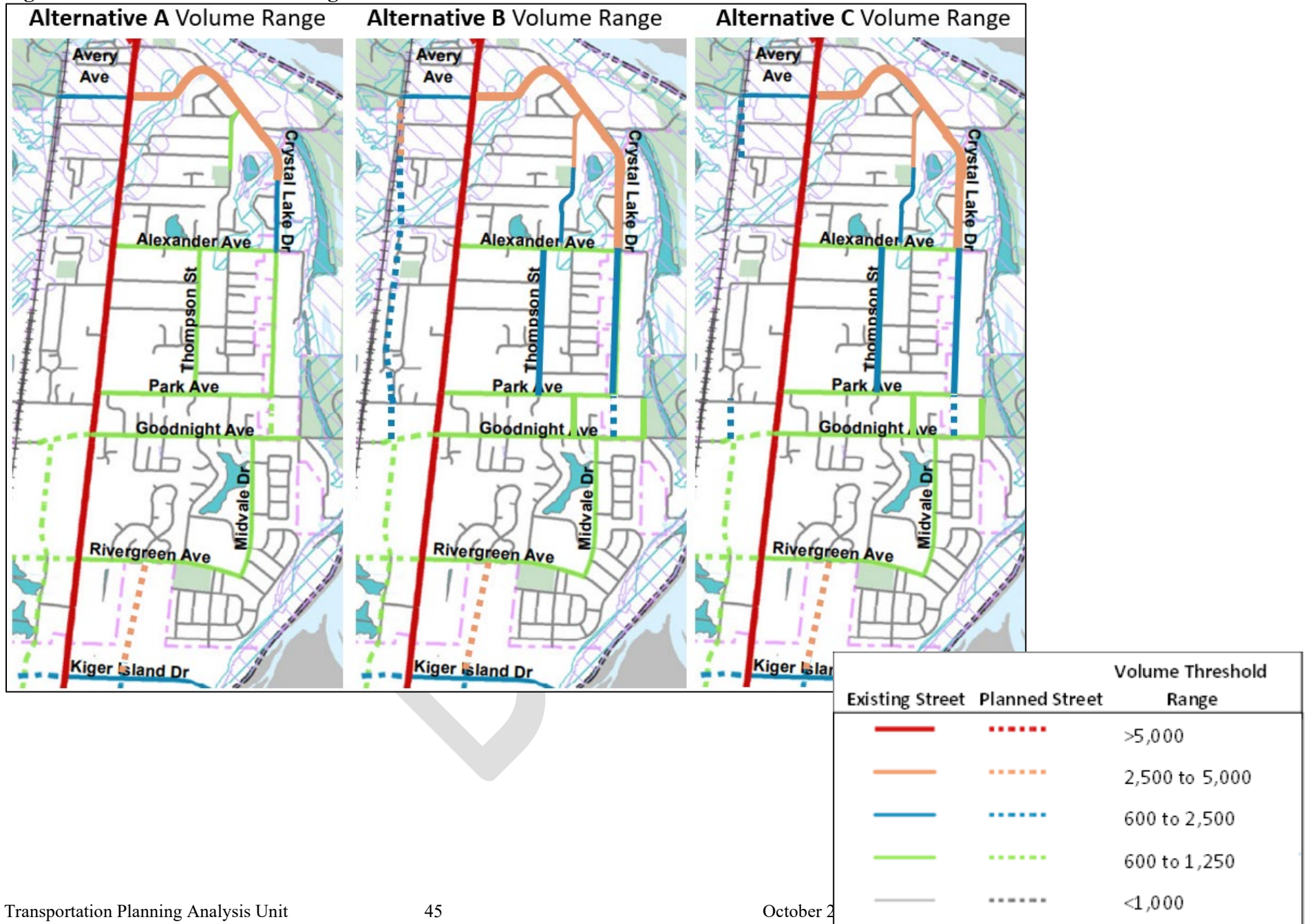
Figure 10- Volume Threshold Ranges Due to Potential Volume Diversion for Build Alternatives
