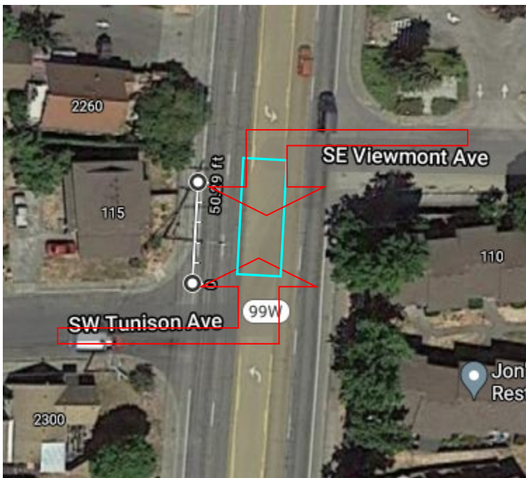
Figure 2: Overlapping Conflict Zone between Viewmont Avenue and Tunison Avenue
