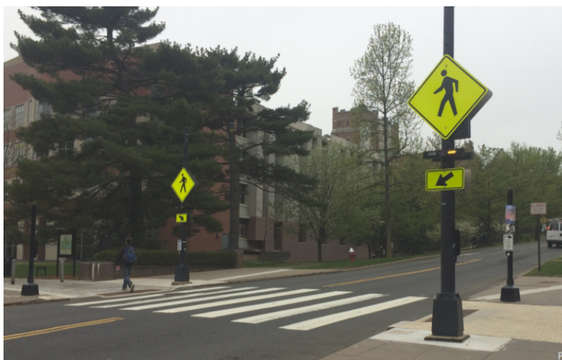
Figure 28: An Example of a Rectangular Rapid Flashing Beacon (RRFB)
