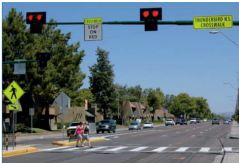
Figure 27: An Example of a Pedestrian Hybrid Beacon (PHB)
