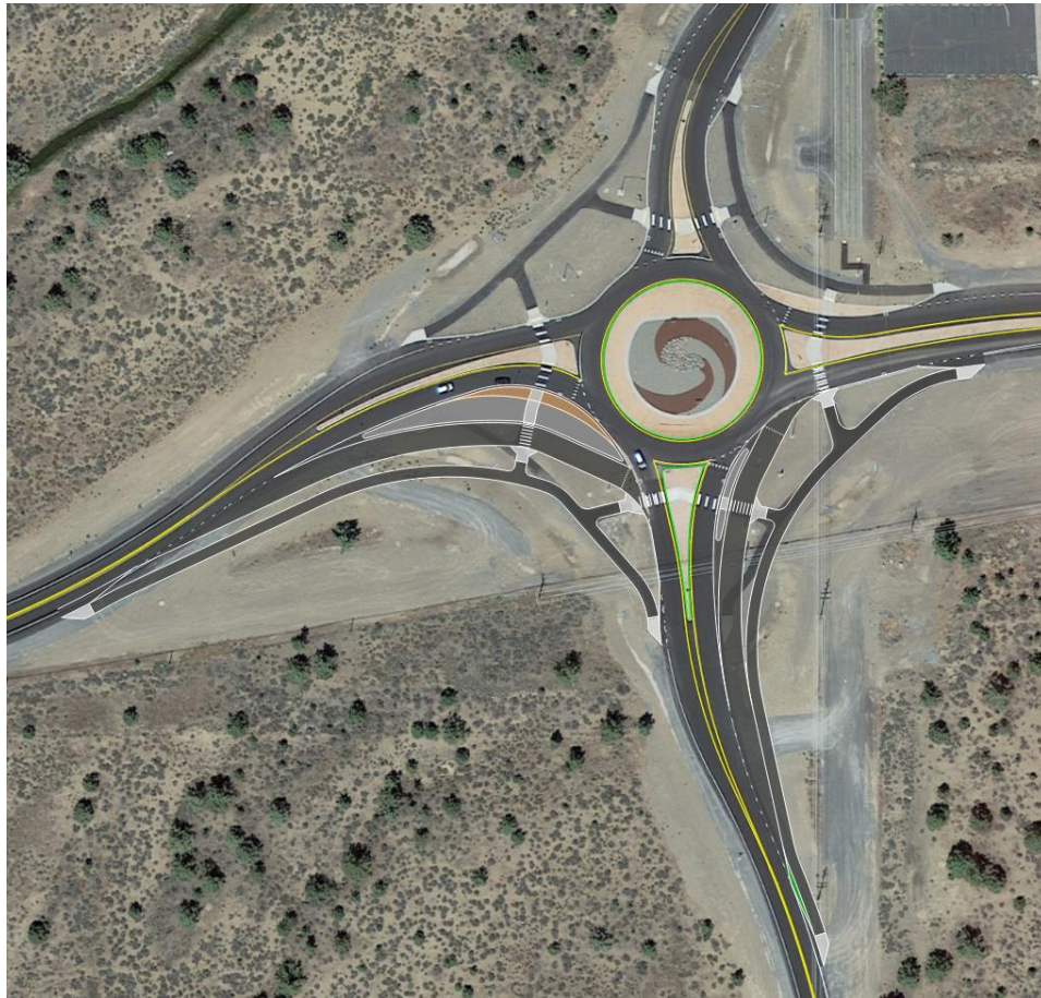
Figure 6. Hamby Road Proposed Slip Lanes
