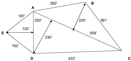
By adding lines AC and AD, irregular shape ABCDE can be broken into three separate triangles. They are ABC, ACD and ADE. Next add the "dashed" height lines for each of the triangles. Measure the resulting heights and bases and you are ready to solve for total area as being the sum of the areas of the three triangles.
