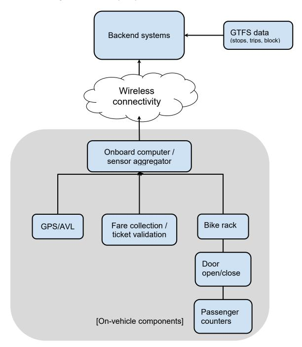
**#2 Stand-alone APC:** APC device or system that may include its own CPU, GPS, and time tracking system. A common wireless connection might be used, or each system may have its own wireless connection.
