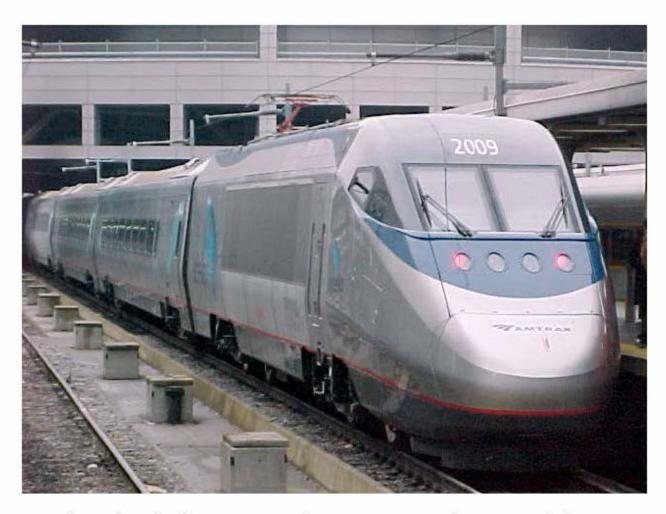
Amtrak Acela - the fastest train in the US. It can reach top speed of 150 mph / 250 kph -- on short sections of track in Rhode Island and Massachusetts. Most of the route has track and overhead wires designed for slower speeds.
