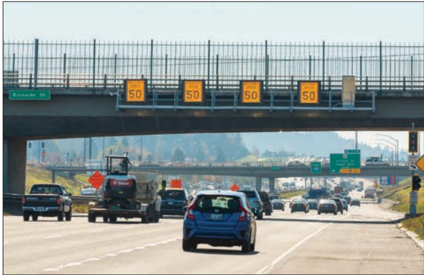
Variable Advisory Speed Signs display speeds based on traffic ahead.
