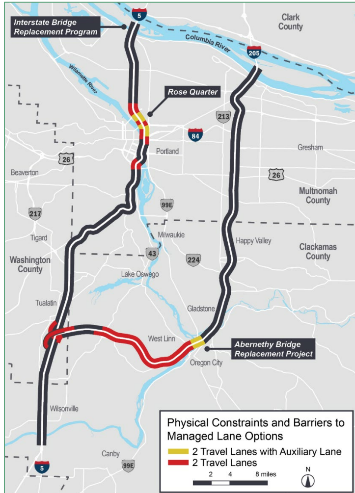
Figure 1: I-5 and I-205 Segments with 2 Travel Lanes
