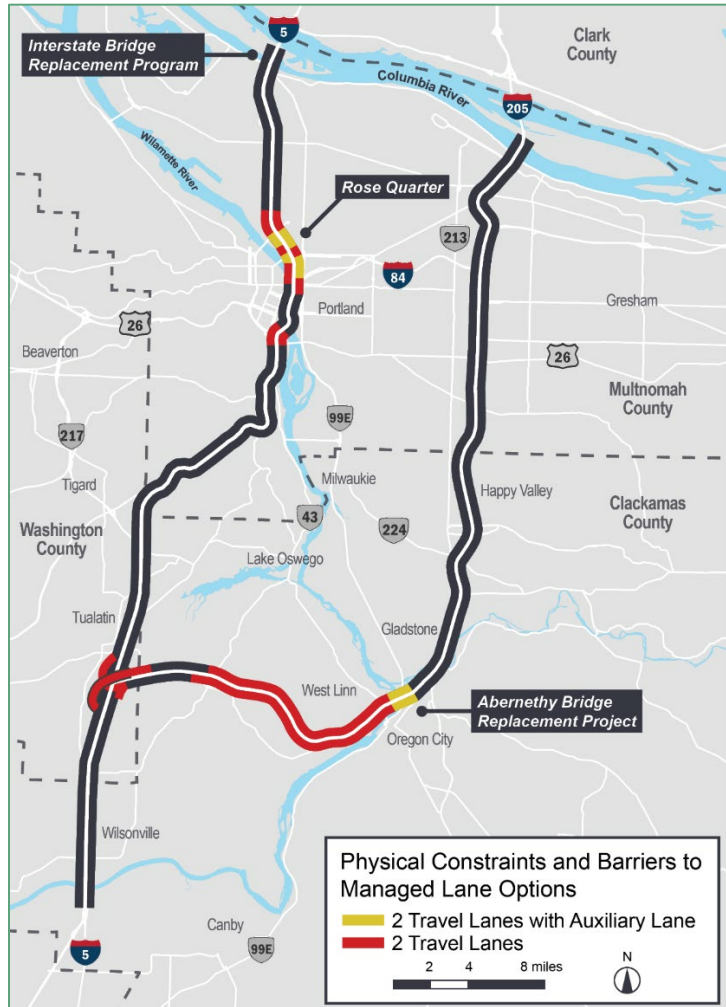
Figure 1: I-5 and I-205 Segments with 2 Travel Lanes
