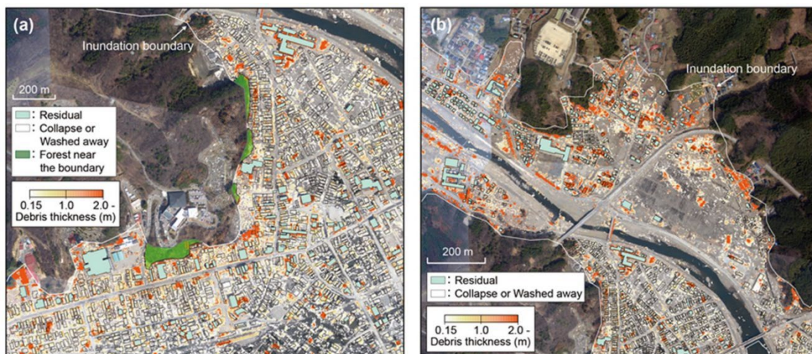
Figure 23. The distribution of tsunami debris in Otsuchi area A, estimated by using a DSM and a DEM with 1 m resolution. (a) An example showing the corrected positions of buildings after the removal of trees at the inundation boundary. (b) The corrected tsunami debris thickness distribution estimated from the difference between the DSM and DEM. (Imai et al., 2022)
