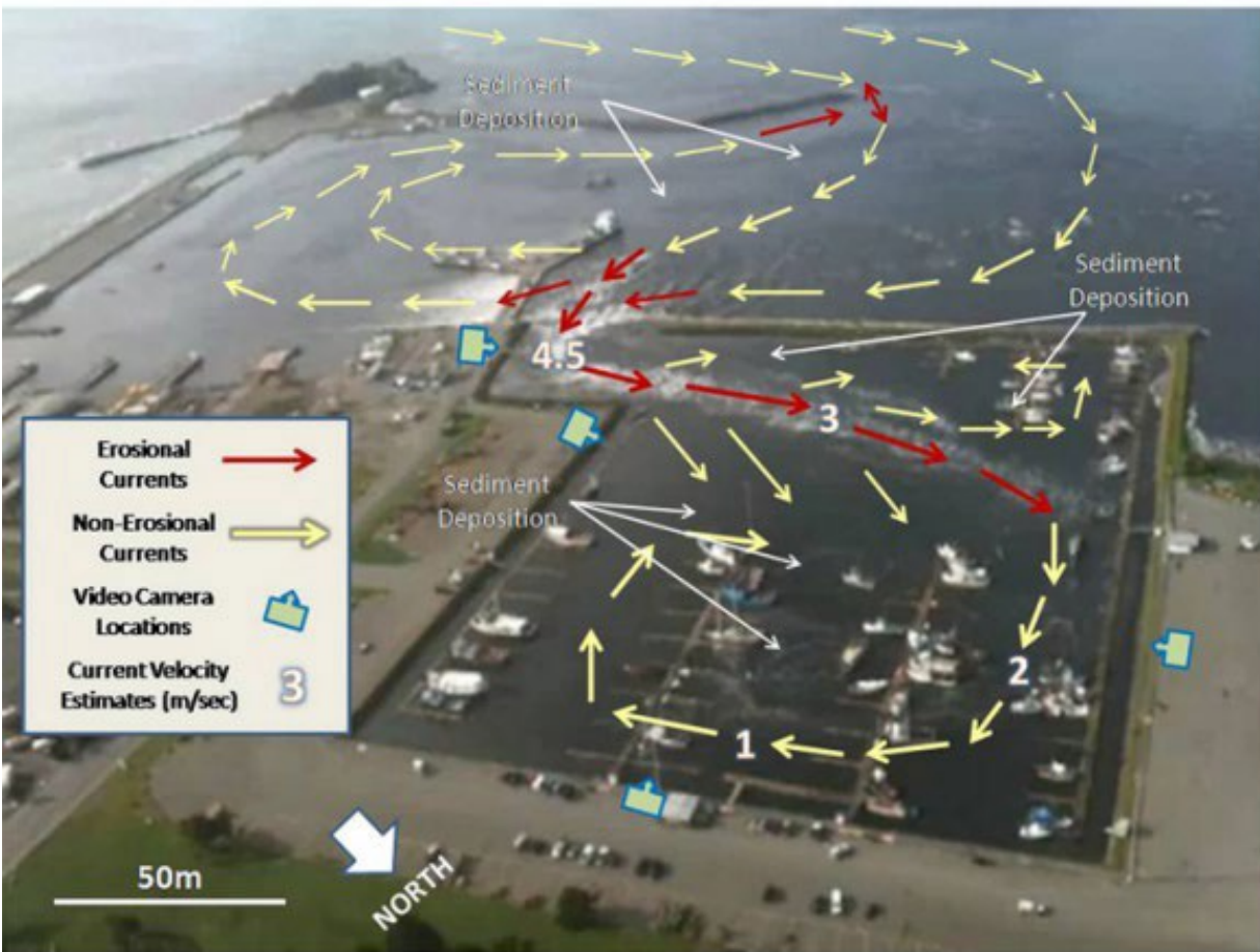
Figure 21. Tsunami flow-regime map for Crescent City Harbor, CA. Current directions and velocities, and areas of sediment erosion and deposition are based on observations of the various (30) ground-level and aerial video, pre- and post-tsunami bathymetry, and sediment analyses. (Wilson et al, 2012)
