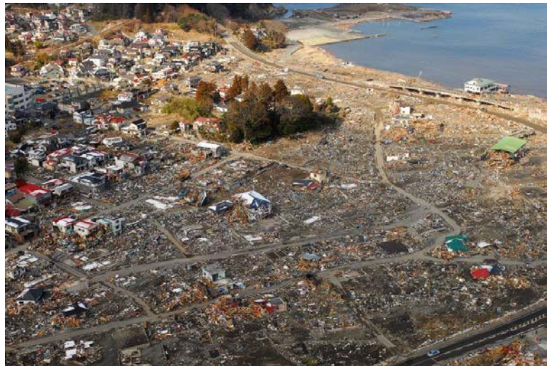
Figure 16. Post-tsunami debris field in a Japanese community after the 2011 Great East Japan tsunami. Note the damaged wood-frame structures pushed to the edge of the inundation area.
